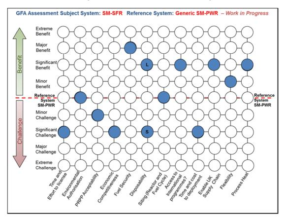
Figure 3: GFA of SM Sodium Cooled Fast Reactor with Generic SM-PWR Reference
