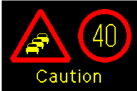
Figure 4F: VMS displaying queue caution information with a reduced mandatory speed limit
