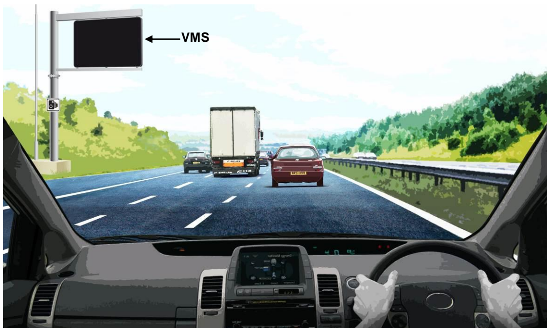
Figure 4B: Illustrative M4 J3 to J12 smart motorway scheme section operating in normal motorway conditions with a blank cantilever mounted VMS
