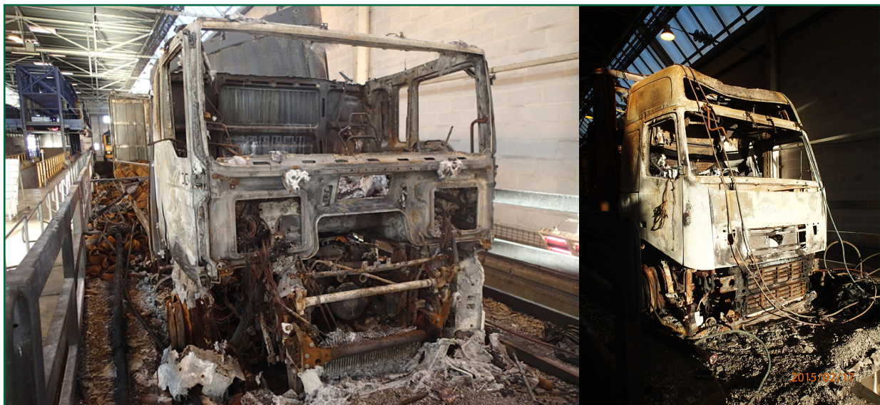
Figure 1: Images of the damage to the two lorries (both still located on the carrier wagons)
