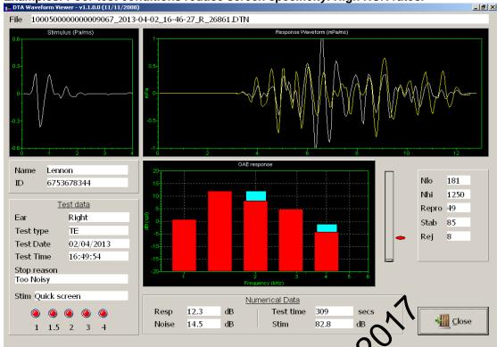
The example above is of a test was allowed to run in noisy conditions to time out. **Nhi** is more than 3 times **Nlo** resulting in a stop reason of "Too Noisy". The stimulus level is within the acceptable range but stimulus stability is only just. This means that while ear piece fit is acceptable, environmental noise levels were too high to report the presence of an AOAE if there was one.
