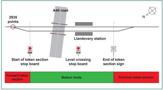
Figure 8: The station limits and single line sections at Llandovery (not to scale)
