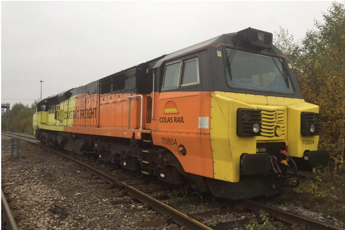
The locomotive derailed at the trap points (photo courtesy of Network Rail)
