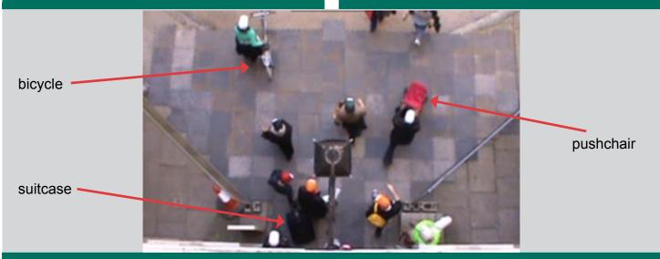
Figure 5: Experimental set-up, 2.4m exit width, without bollard array with 60% encumbrance level.
