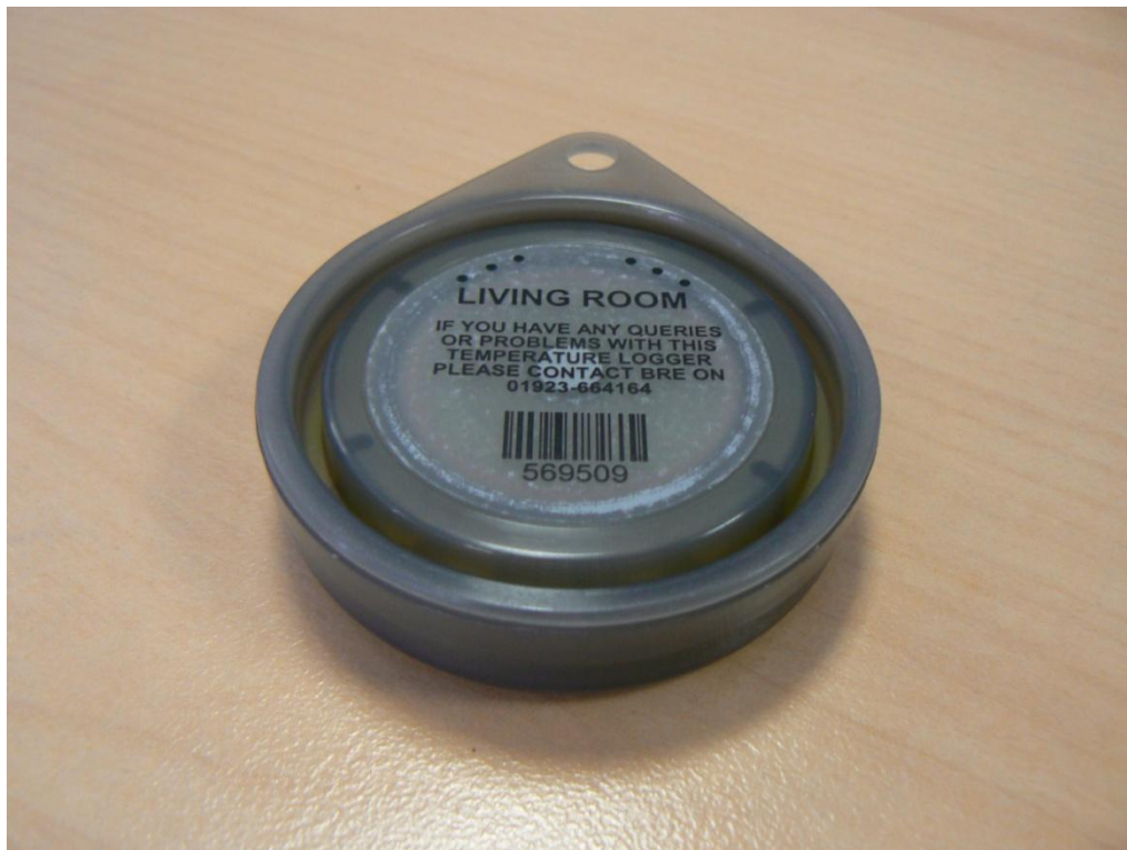
Figure 1: Modified Tinytag Transit 2 temperature logger.
