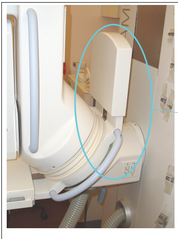
Figure 42 Siemens Mammomat 3000 swivelling bucky.
