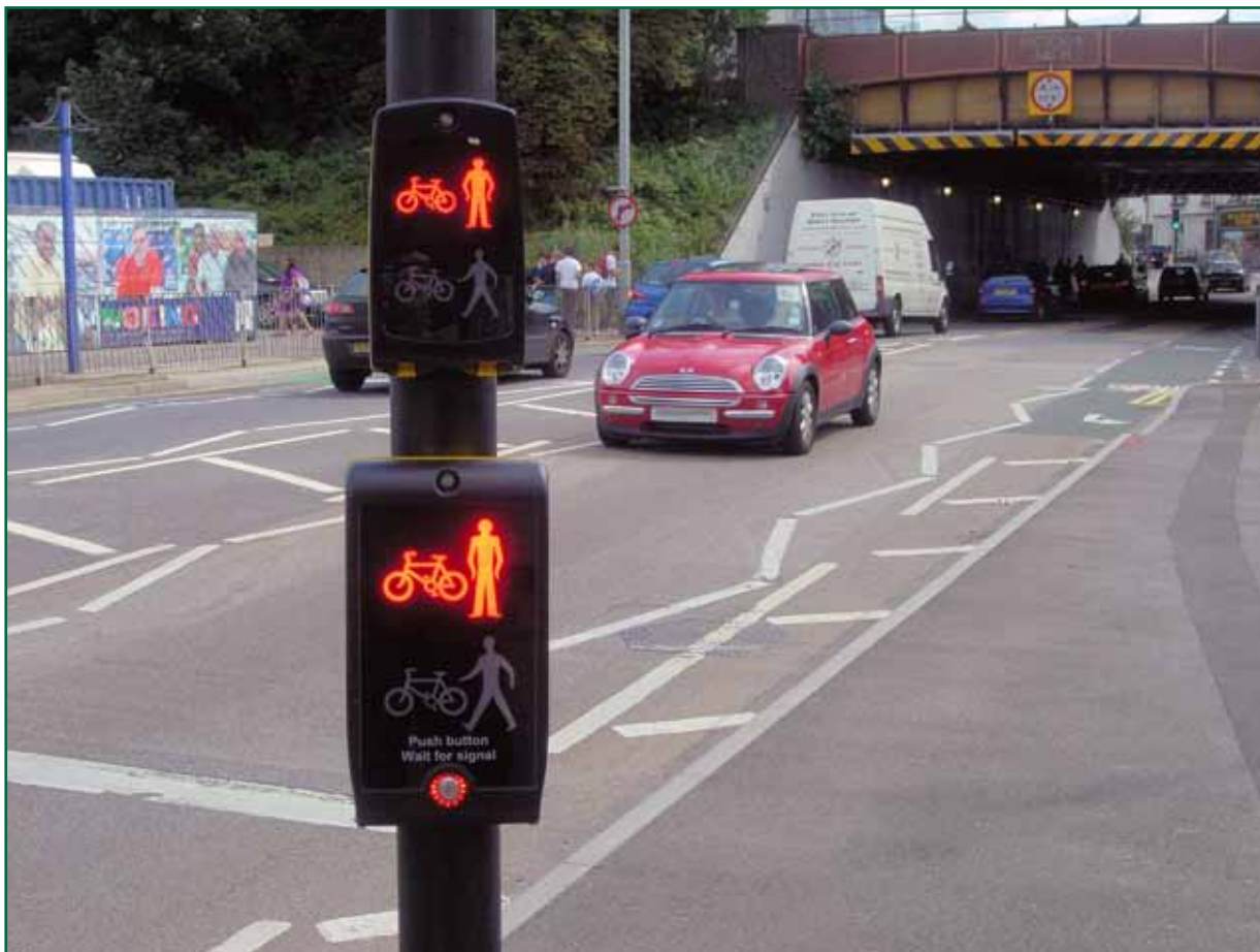
Figure F1: Puffin crossing showing orientation of nearside lights relative to oncoming traffic
