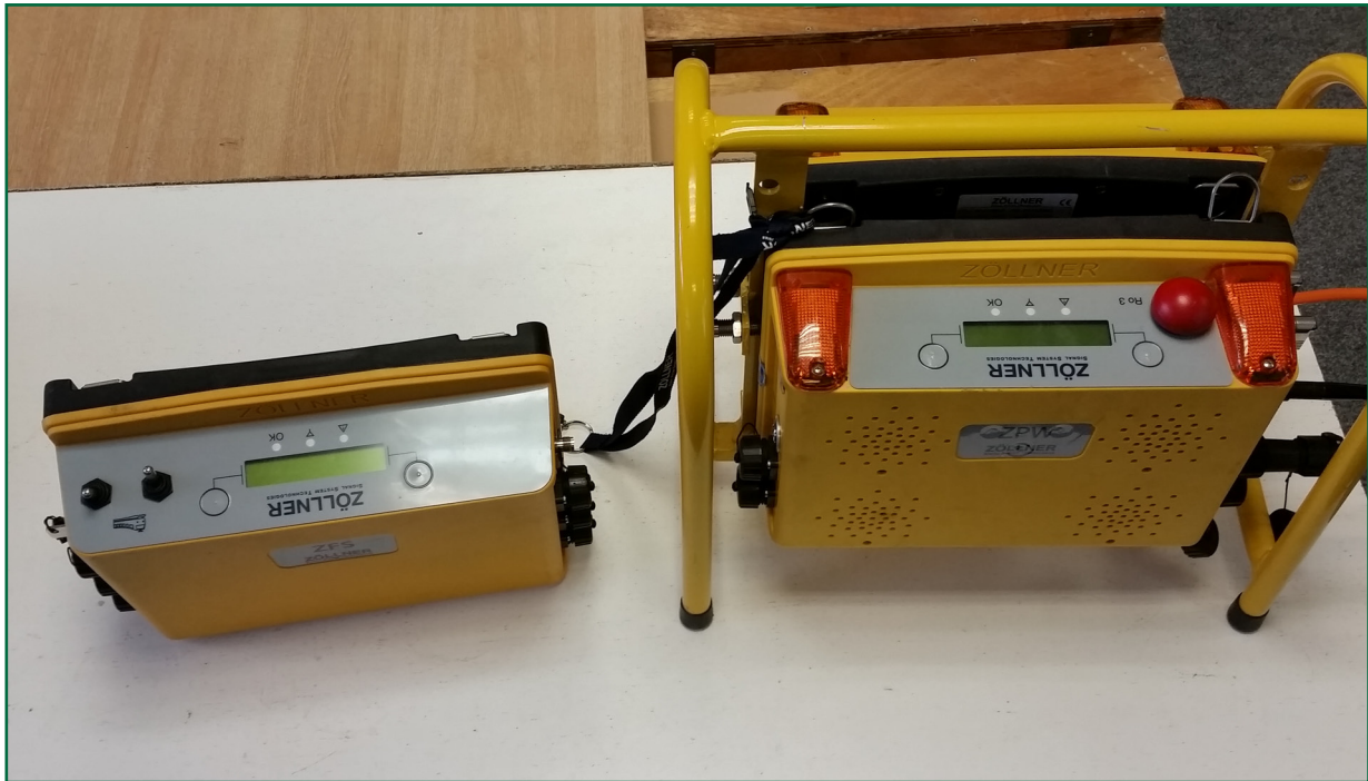
Figure 12: Zöllner LOWS version 2 ZFS radio transmitter and ZPW control unit
