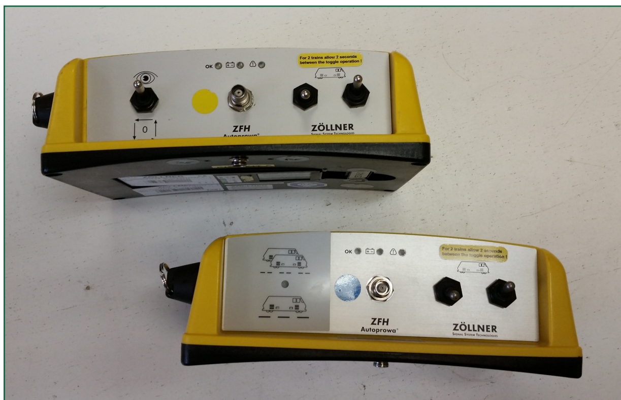
Figure 11: ZFH version 1.4 lookout unit (left) and ZFH version 1.5 lookout unit (right); note absence of vigilance switch on version 1.5 unit
