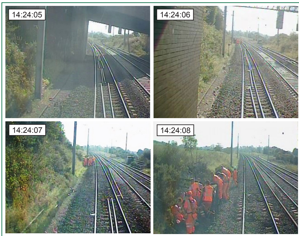
Figure 9: Images of workgroup from forward-facing CCTV camera fitted to train 1M97 while approaching under the A5105 bridge (courtesy of FTPE). Clock times are based on OTDR data.
