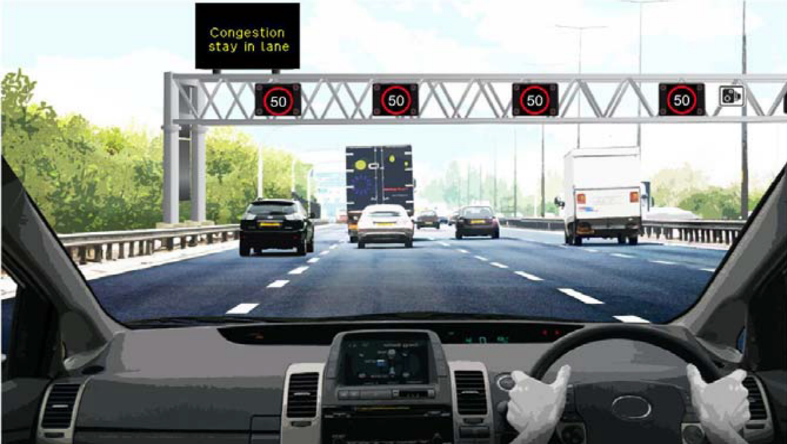
Figure 3G: Illustrative MM-ALR section operating with Variable Mandatory Speed Limits
