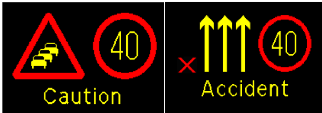
Figure 3J: Variable Message Sign displaying queue caution information with a reduced mandatory speed limit and a lane closure red X with reduced mandatory speed limit
