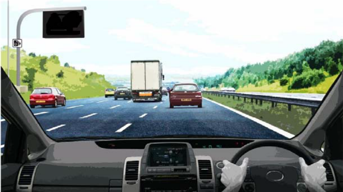
Figure 3D: Illustrative MM-ALR section operating in normal motorway conditions with a blank verge mounted Variable Message Sign
