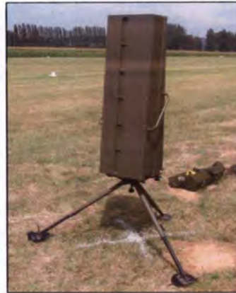
Figure 6 – Ground Radar Unit (GRU)
