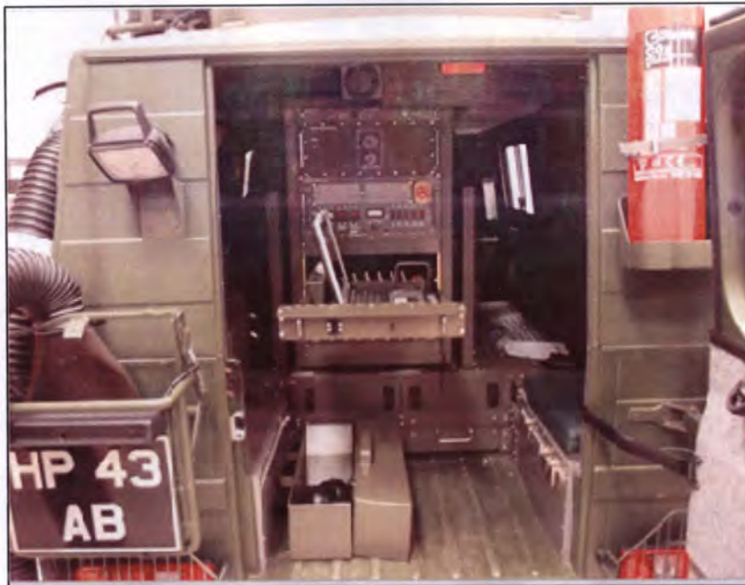
Figure 7 - The Portable Air Vehicle Test Equipment (PATE)
