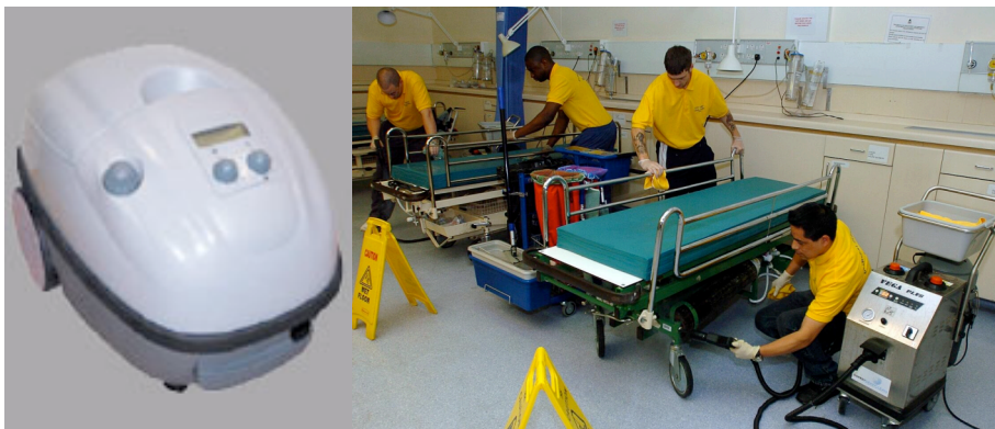
Figures 6 and 7: The steam and vacuum cleaning tools in use in University College London Hospital during the current study.
