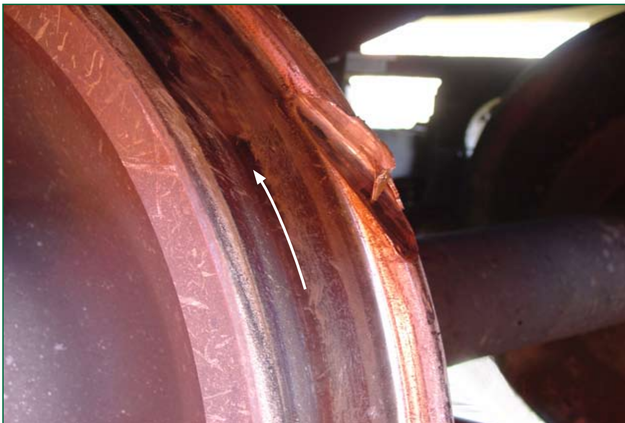
Figure 16: Left trailing wheel on leading bogie of wagon HTA 310724 showing deep flange damage.
