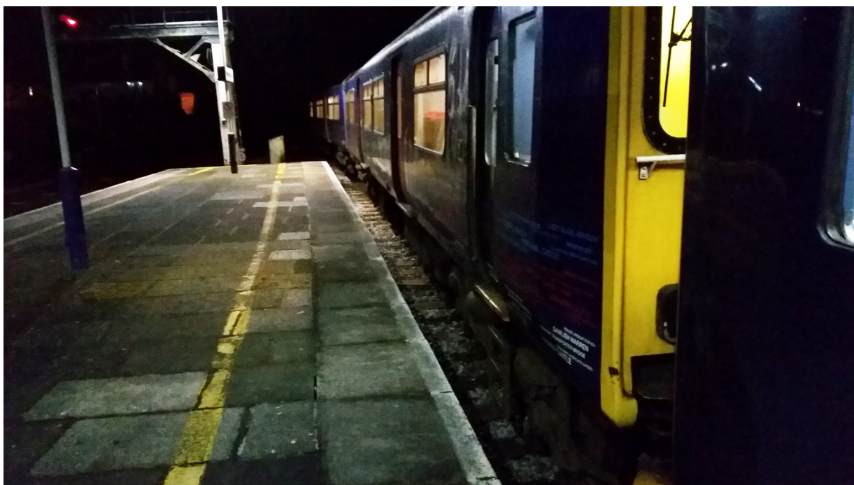
Figure 10: Gap between the third vehicle of train 2E68 and the platform edge
