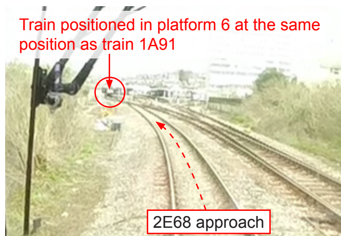
Figure 12: Platforms 3, 4, 5 and 6 become visible from about 135 metres from the station (image courtesy of GWR)
