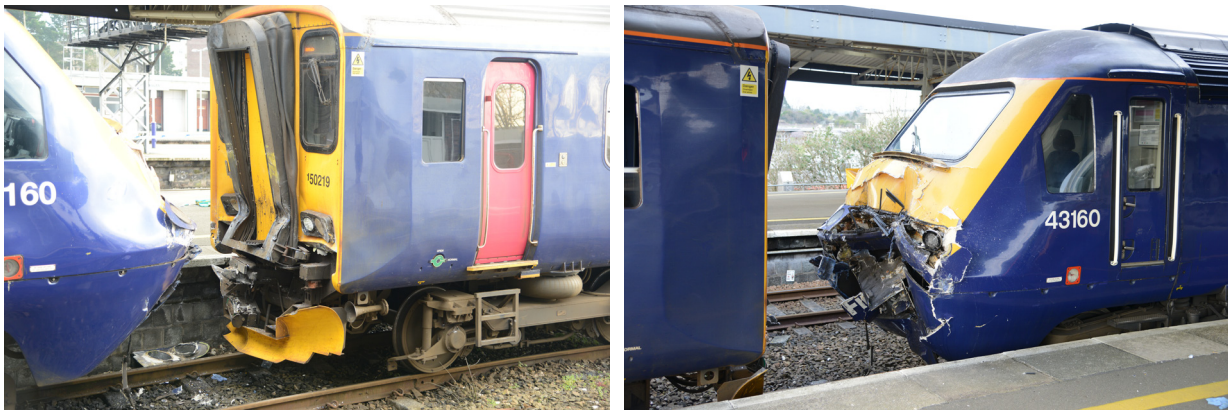
Figure 2: Damage to train 2E68 (left image) and train 1A91 (right image)
