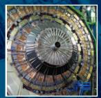
CMS: front view of the innermost endcap disc. (Courtesy CERN)
