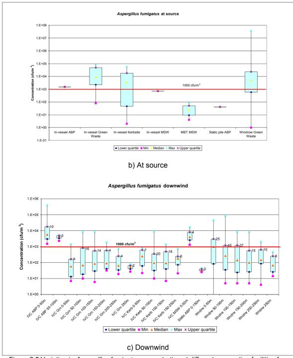
Figure 2.5 Variation in *Aspergillus fumigatus* concentration at different composting facilities for a) upwind, b) at source (0–10 m from source) and c) downwind (>10 m downwind).
