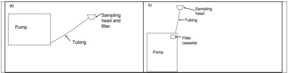
Figure 2.2 The schematic diagrams of a) the SKC sampling equipment, and b) the novel sampling equipment, showing the location of the pumps, tubing, filters and sampling heads.
