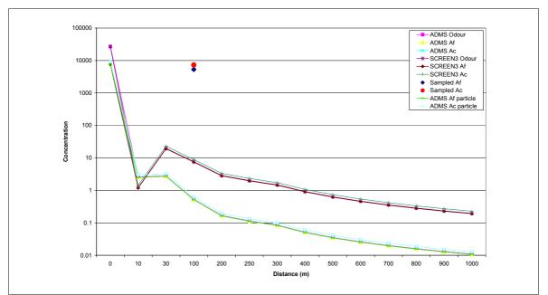
Figure 2.7 Downwind SCREEN3 and ADMS 3.3 predicted concentrations of odour, *Aspergillus fumigatus* and actinomycetes for Site B. Note: Bioaerosol concentrations are in  $cfu/m^3$  and odour concentrations are in  $ou_E/m^3$ . The x axis is on a nonlinear scale.
