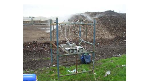
Figure 2.1 The two types of samplers with the pumps and sampling boxes on the lower platform for easy access, and the sampling heads at the end of the tygon tubing at a height of 1.8 m. The compost windrow can be seen in the background.
