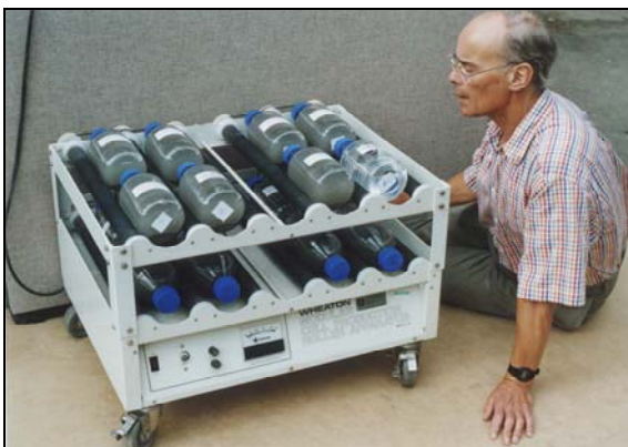
Plate 9 Roller table in operation
