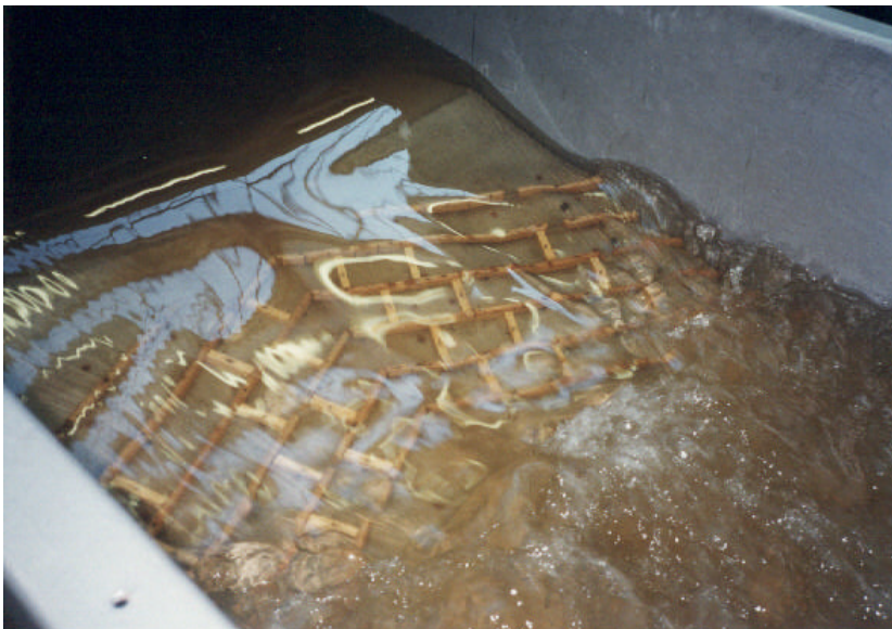
Figure 2.1: Model of Flat-V weir, Moors River, Hurn, Dorset
