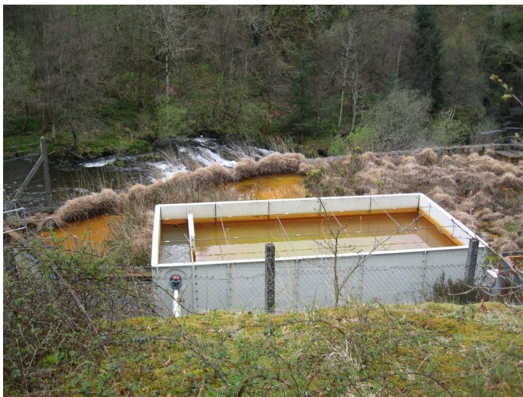
Figure 6. Pilot-scale reactor for remediation of discharge from Adit No. 6 at Cwm Rheidol
