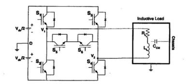
Figure 3.3: Schematic Diagram of the Proposed Single Phase Inverter Driving a Passive Load
