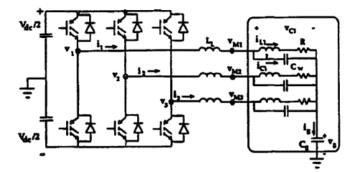
Figure 2.9: Illustration of Common Mode EMI Generation in a Typical Three Phase PWM Drive System
