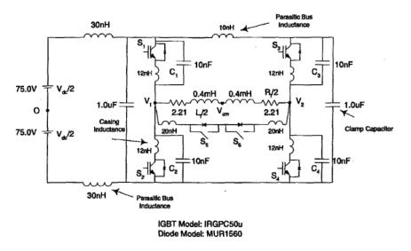
Figure 4.7: Simulation Model of Laboratory Prototype Inverter with Proposed Topology
