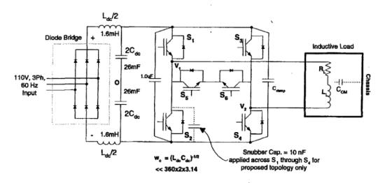
Figure B.1: Schematic Power Circuit Diagram for Laboratory Prototype Inverter
