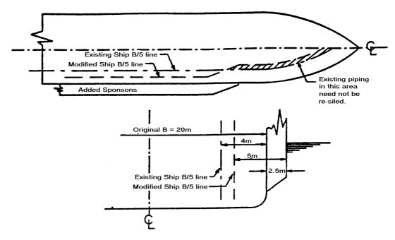
(Note: the phrase B/5 refers to the transverse damage extent required by the 1994 or the 2000 HSC Code for side damages).
