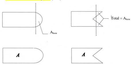
Figure 4.4.1: Plan view of two different craft styles
