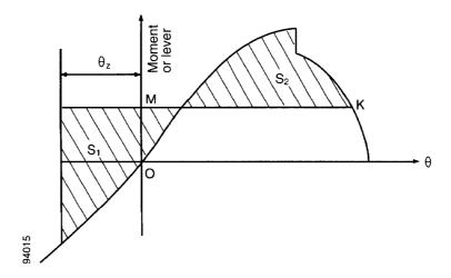
Figure 1 - Static stability curve
