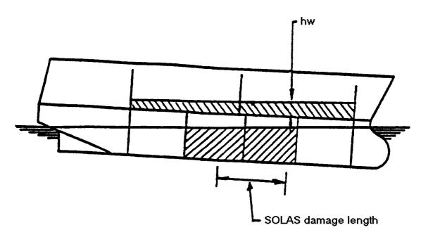
(Note: SOLAS damage length refers to side damage length of HSC / DSC Code.)
