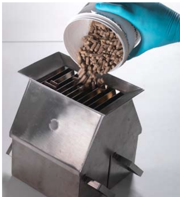
Figure 4: Rigorous sample preparation contributes to high quality measurement. A riffle splitter can provide representative subsamples of fragmented solids such as this animal feed product.
