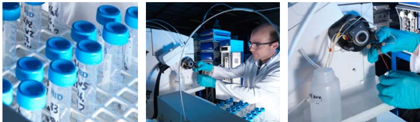
Figure 7: Volker Nischwitz is using a state-of-the-art field flow fractionator with ICP-MS to perform size-based element speciation on engineered nanoparticles.
