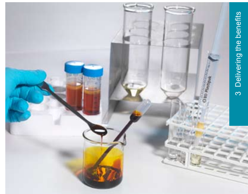
Figure 5: Extraction of dimethyl yellow dye from a complex oleoresin product. The sample as received was a viscous liquid (glass beaker). After mixing with suitable solvents, any dimethyl yellow dye present is found mainly in the top layer (centre left). This extraction step is repeated, the top layers are combined in a large glass tube, and the solvents are removed by accelerated evaporation (centre right). The residue is redissolved and further purified by gel permeation chromatography (not shown) and solid phase extraction with silica (far right). Subsequently, the extract is again evaporated and redissolved, then transferred to an autosampler vial for analysis by LC-MS/MS.
