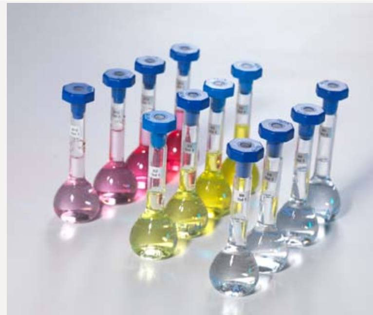
Figure 6: Solutions containing accurately known concentrations of vitamins B2 (yellow), B6 (clear) and B12 (pink) are among the calibrators needed to make quantitative micronutrient measurements.
