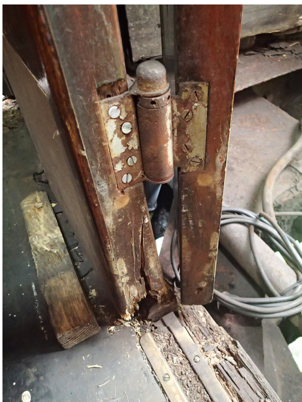
Figures 16 to 19: The damage to the toilet cubicle frame and door of carriage 4805
