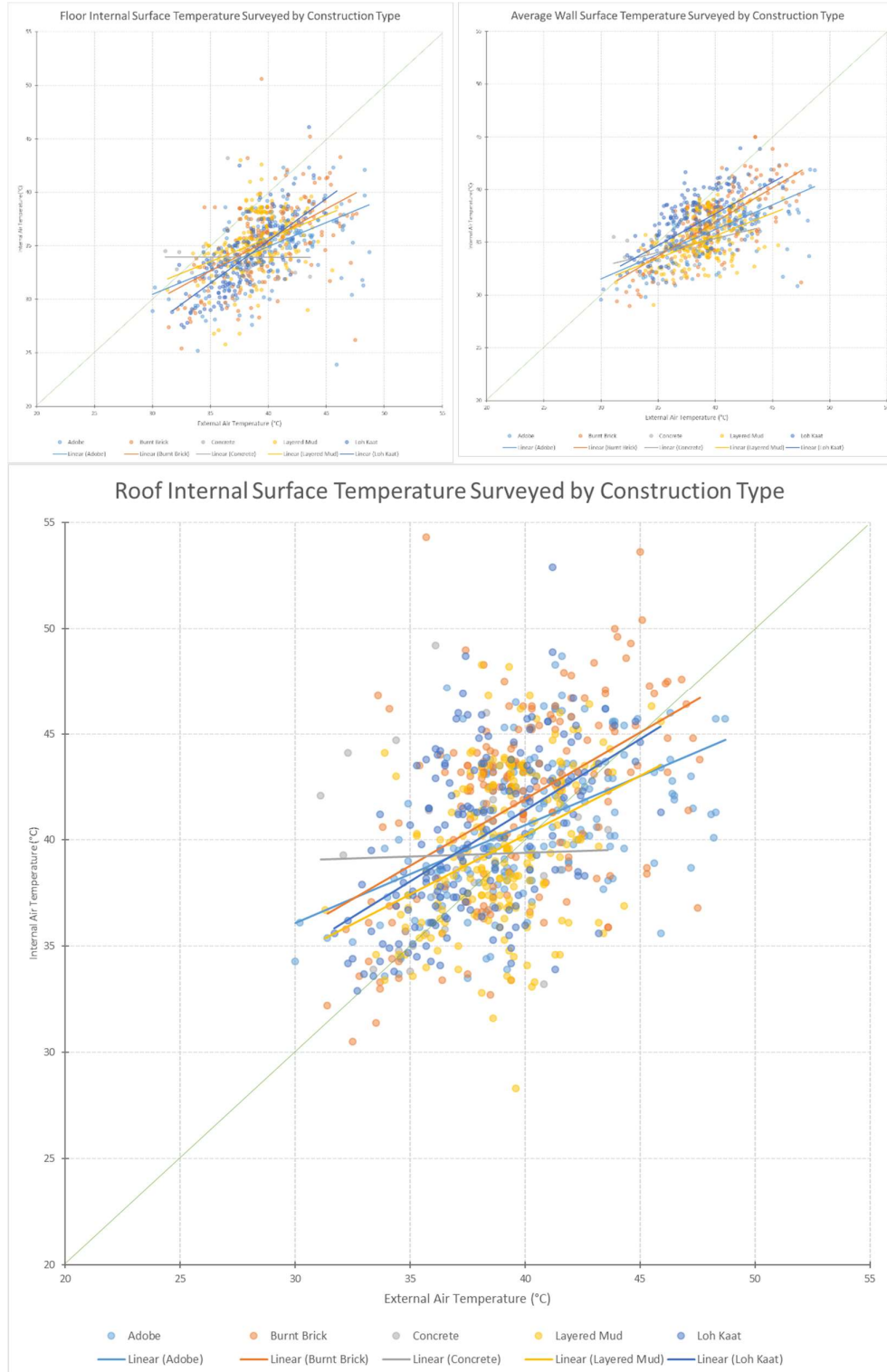
Figure 4 Internal surface temperatures surveyed by type against the corresponding external shade temperature surveyed.
