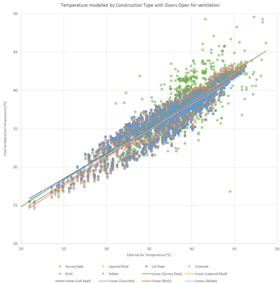
Figure 13 Comparison of modelled internal operative versus external air temperatures for each construction type with ventilation provided by open doors
