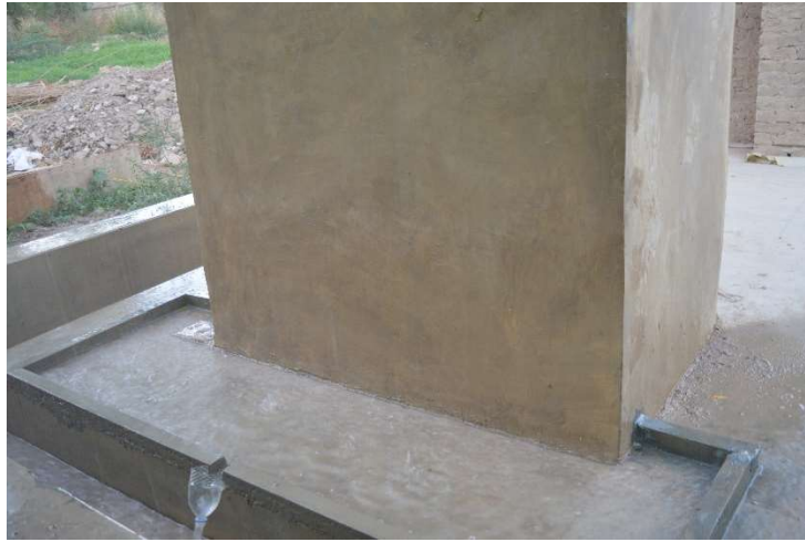
Figure 7. Sample collection and flow accumulating pit
