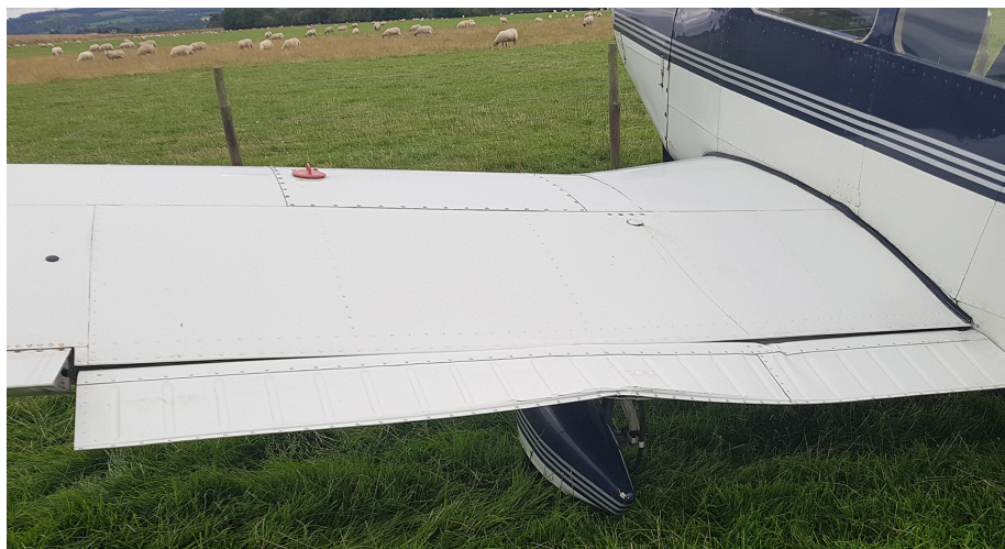
Figure 1 Damage to left flap
