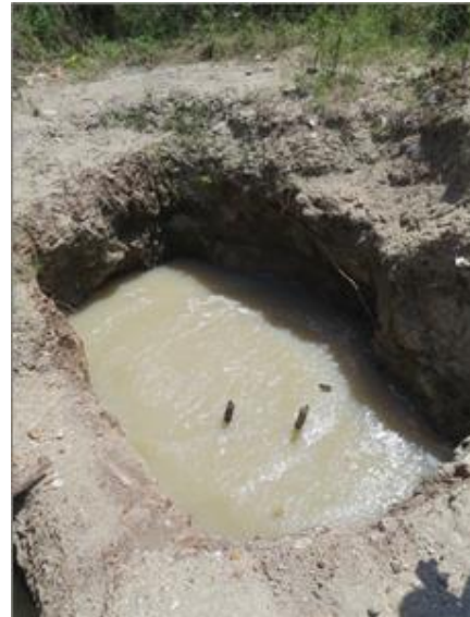
Figure 17: Flooded Shaft in Morita
