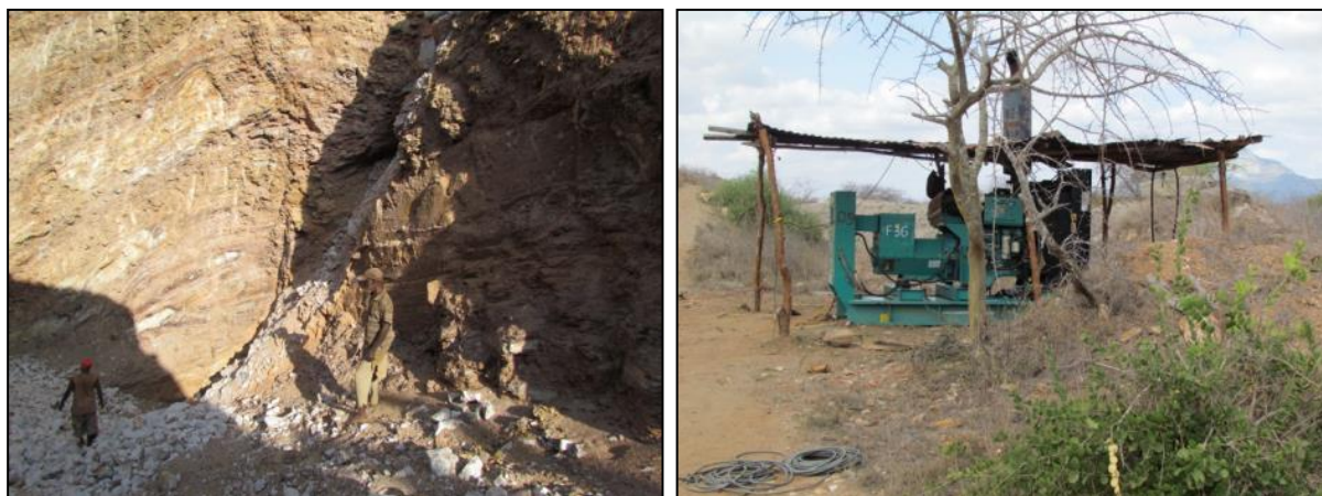
Figure A49: Considerable investment is required to access deeper and potentially more lucrative deeper deposits, including (left) rental of excavators to follow promising shear zones from the surface; and (right) large generators needed to power jackhammers and other small equipment
