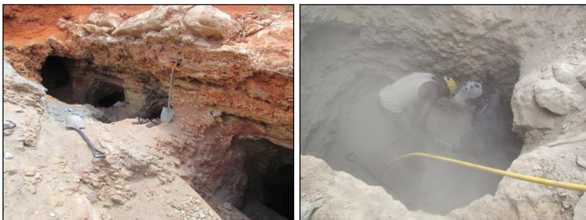
Figure A52: (Top left) Adits providing access to a deeper gallery of interconnected tunnels; (Top right) Dust exposure during dry rock breaking with jackhammers presents a serious health risk; (Bottom left) Living conditions at one of the mine sites; (Bottom right) A diversity of wildlife can be found across the area
