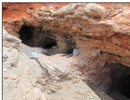
Figure 20: A series of adits (mine entrances) are excavated to access the same gemstone-bearing shear zone
