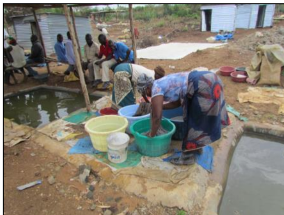
Figure 10: Sluice mats are washed by women to recover concentrate before amalgamation in nearby impoundments
