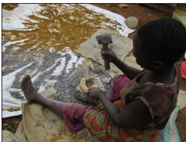
Figure A35: Top: Ore is Crushed (top left) Following by Grinding in Octagonal Mills (top right). Centre: Milled Ore is Poured with Water Over Crude Washing Tables where Concentrate (heavy minerals including gold) is Trapped in Mats (centre left). Mats are Carefully Washed in Large Basins to Collect Concentrate. Bottom: Amalgamation is Performed in Nearby Impoundments (bottom left) and the Resulting Doré is Burnt by Traders in Small Charcoal Stoves to Recover the Gold (bottom right).
