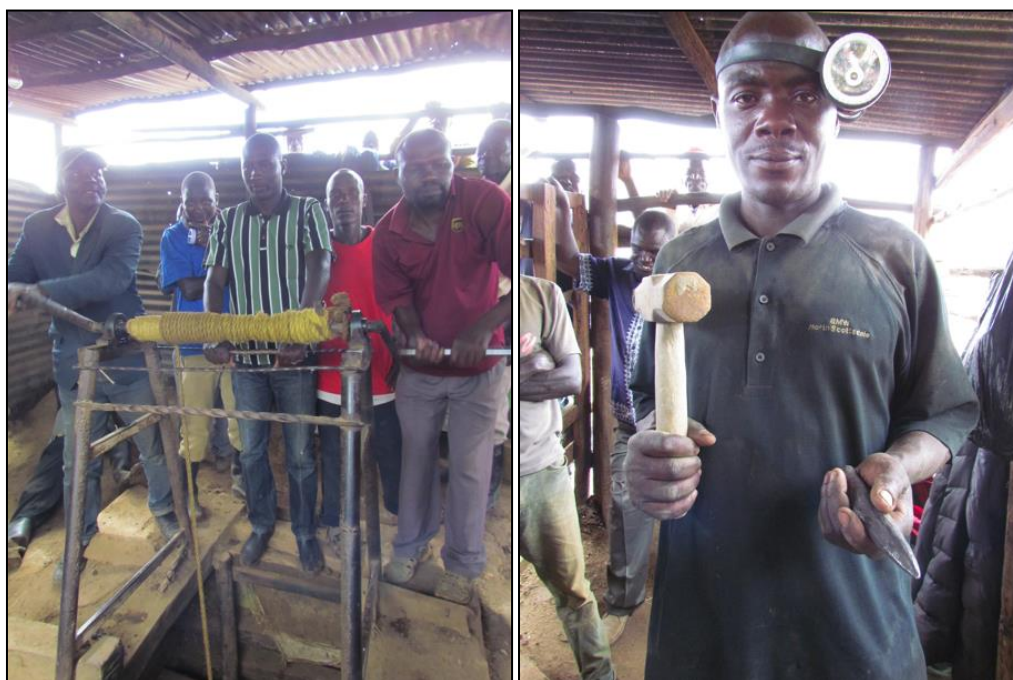
Figure A34: (left) Miners haul up sacks of ore from depth using a winch; (right) Most miners rely on small hammers, chisels and a headlamp
