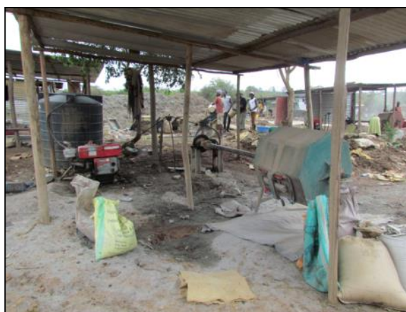
Figure A35: Top: Ore is Crushed (top left) Following by Grinding in Octagonal Mills (top right). Centre: Milled Ore is Poured with Water Over Crude Washing Tables where Concentrate (heavy minerals including gold) is Trapped in Mats (centre left). Mats are Carefully Washed in Large Basins to Collect Concentrate. Bottom: Amalgamation is Performed in Nearby Impoundments (bottom left) and the Resulting Doré is Burnt by Traders in Small Charcoal Stoves to Recover the Gold (bottom right).
