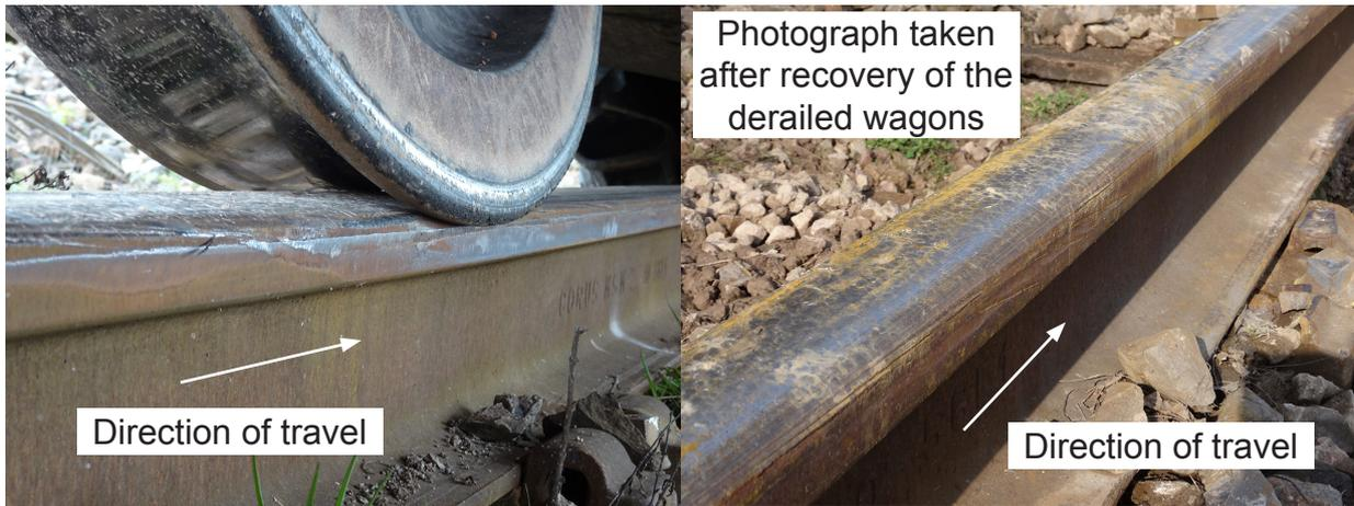
Figure 9: Drop-in marks on the gauge corner of the left-hand rail at bearer nos. -2 and -4 (courtesy Network Rail)
