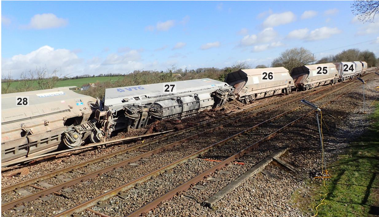
Figure 2: General view of accident site, showing the numbering of the wagons from the front of the train
