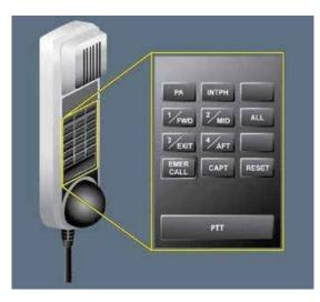
**Figure 7** Interphone communication handset showing keypad
