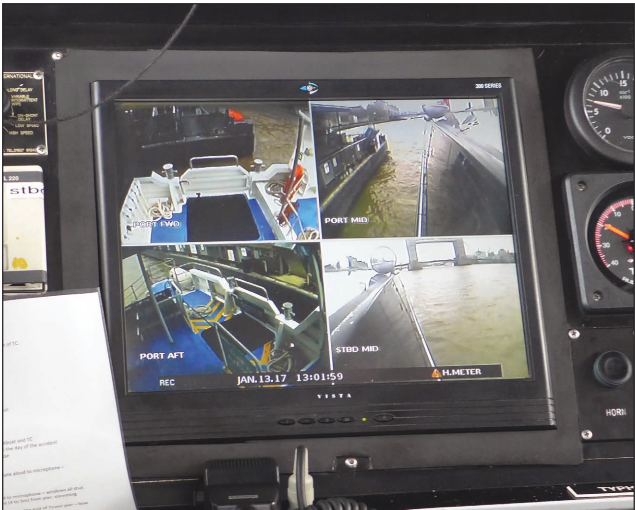
Figure 15: Typhoon Clipper's wheelhouse CCTV display (during the reconstruction) showing the display settings at the time of the accident
