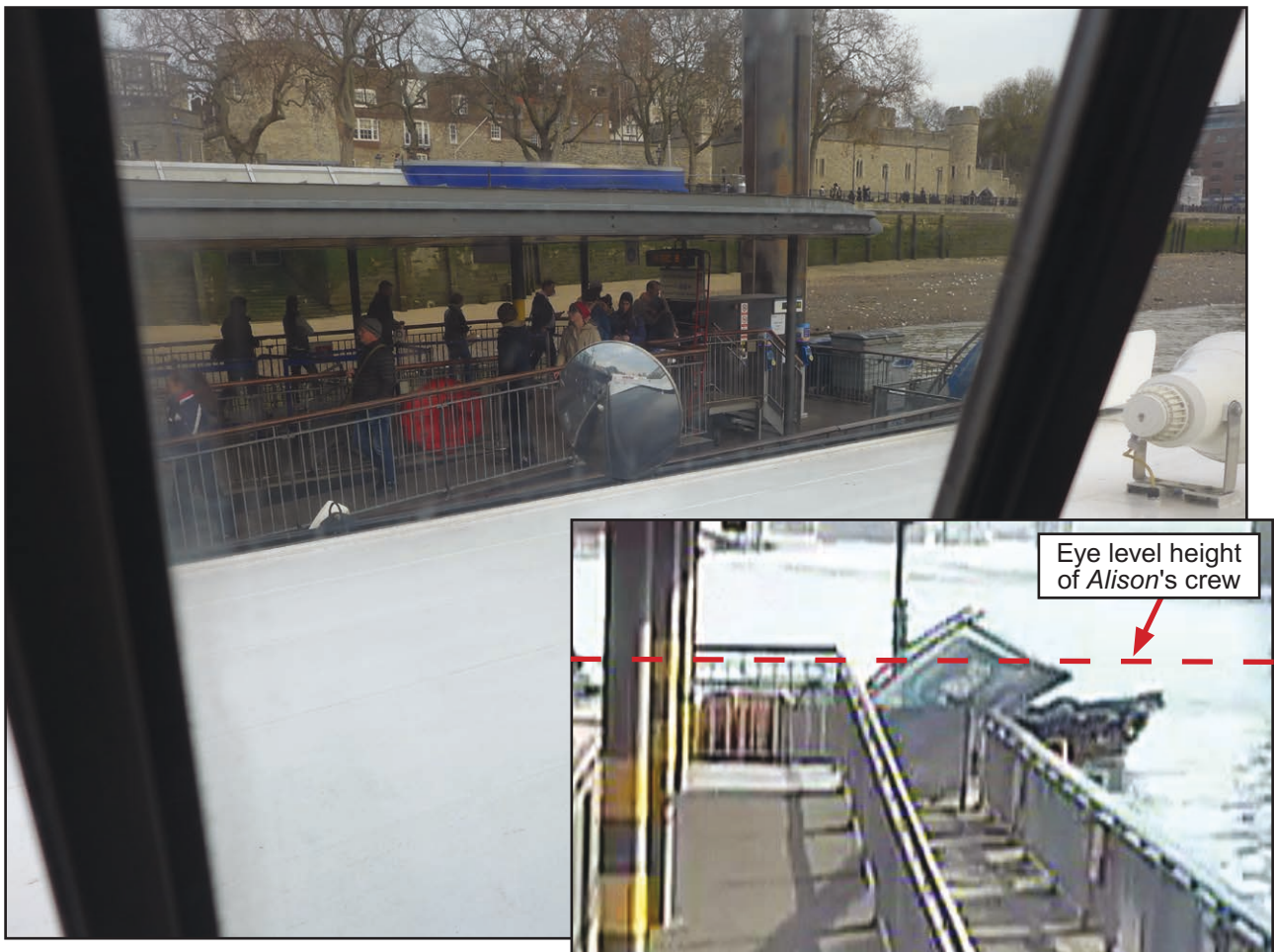
Figure 21: View of the pier from Typhoon Clipper 's wheelhouse (during reconstruction) and inset analysis of height of Alison when close by the pier
