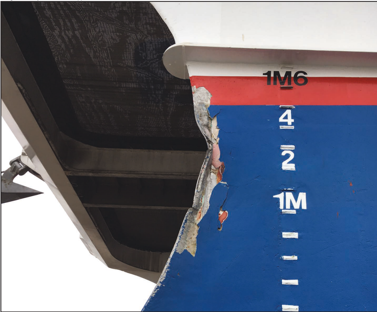
Figure 10: Damage to Typhoon Clipper's port stem
