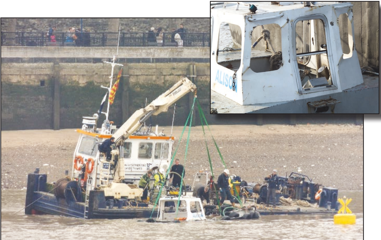
Figure 11: Recovery of Alison off the riverbed with inset detail of its superstructure damage
