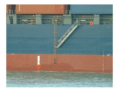
During the pilot transfer the supervising ship's officer should be in direct contact with the bridge. The ship should maintain steerage way at speed that allows the pilot vessel to remain comfortably alongside and should not stop or reverse engines except in an emergency or when requested by the pilot boat Coxswain.
