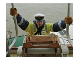
The Deckhand should be secured by a life line to Hadrian's Rail whilst on deck, without the line restricting his freedom of movement. When leaving the cabin, the Deckhand, followed by the Pilot, should pass along the outboard side of the cabin to the boarding position. The Pilot should take all necessary precautions, and consider the use of the Hadrian's Rail, when on he deck of the pilot boat.
