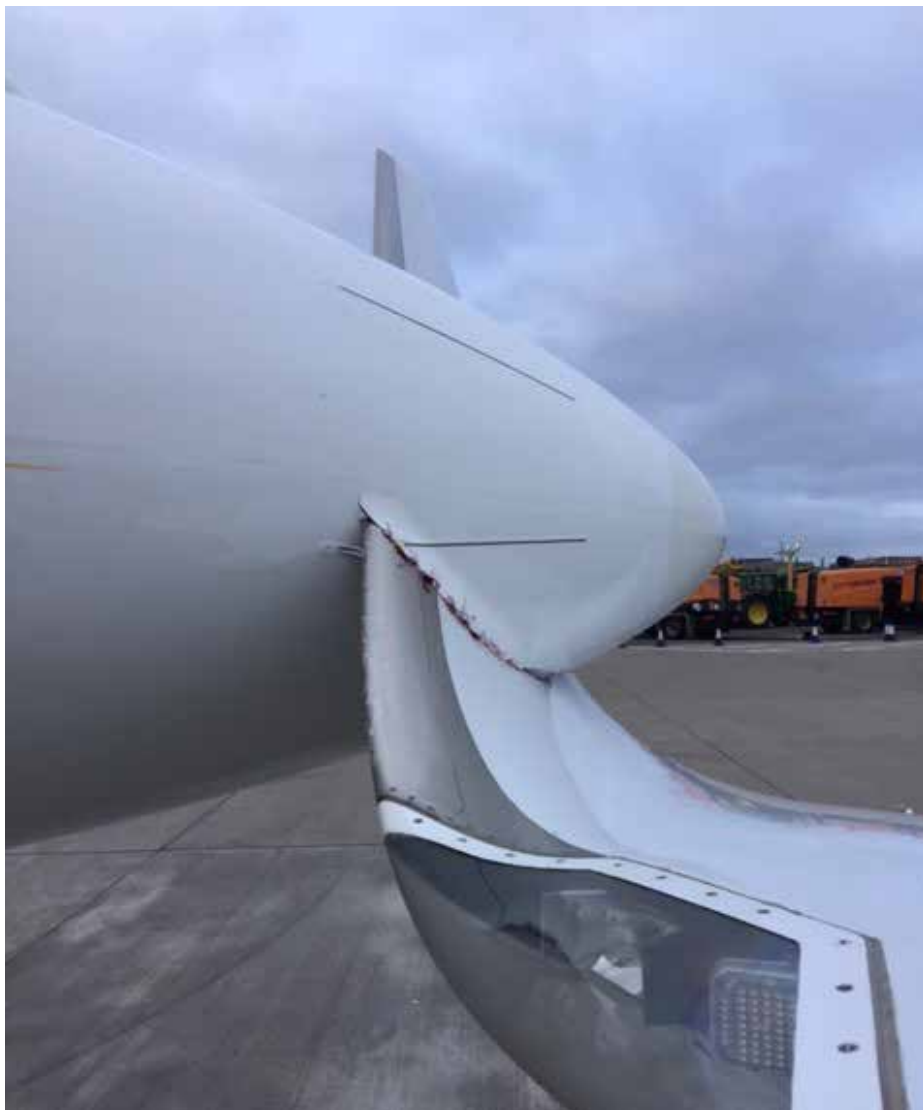
Figure 3 Damage caused by the collision
