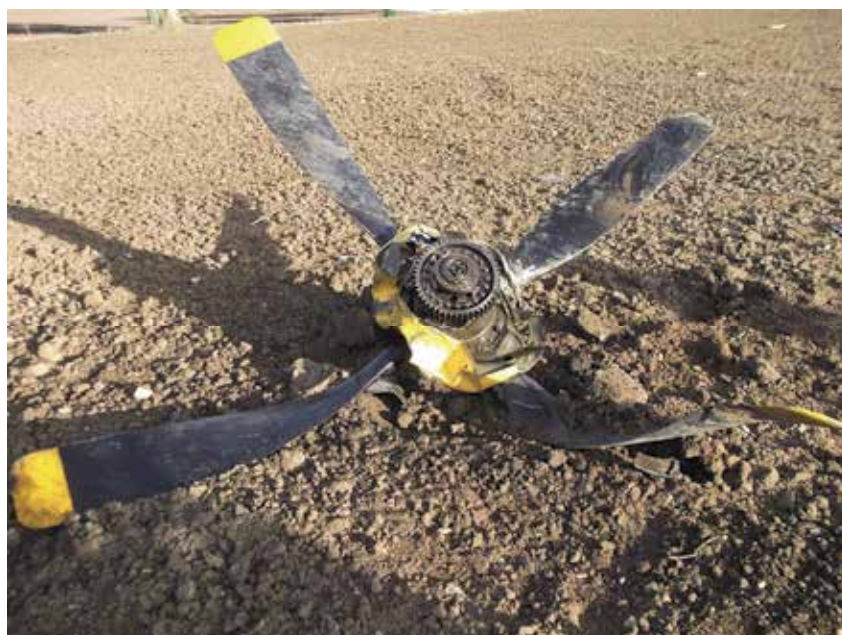
Figure 5 (right) Propeller damage
