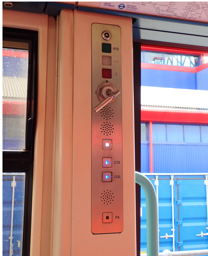
Figure 7: Door Control Panel on a DLR car
