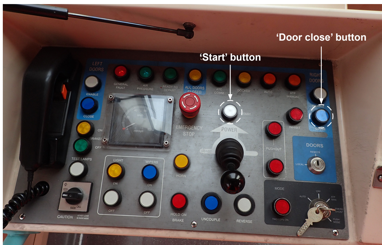
Figure 6: Controls provided at the EDP on a DLR car. The 'Door Close' and 'Start' buttons are indicated.
