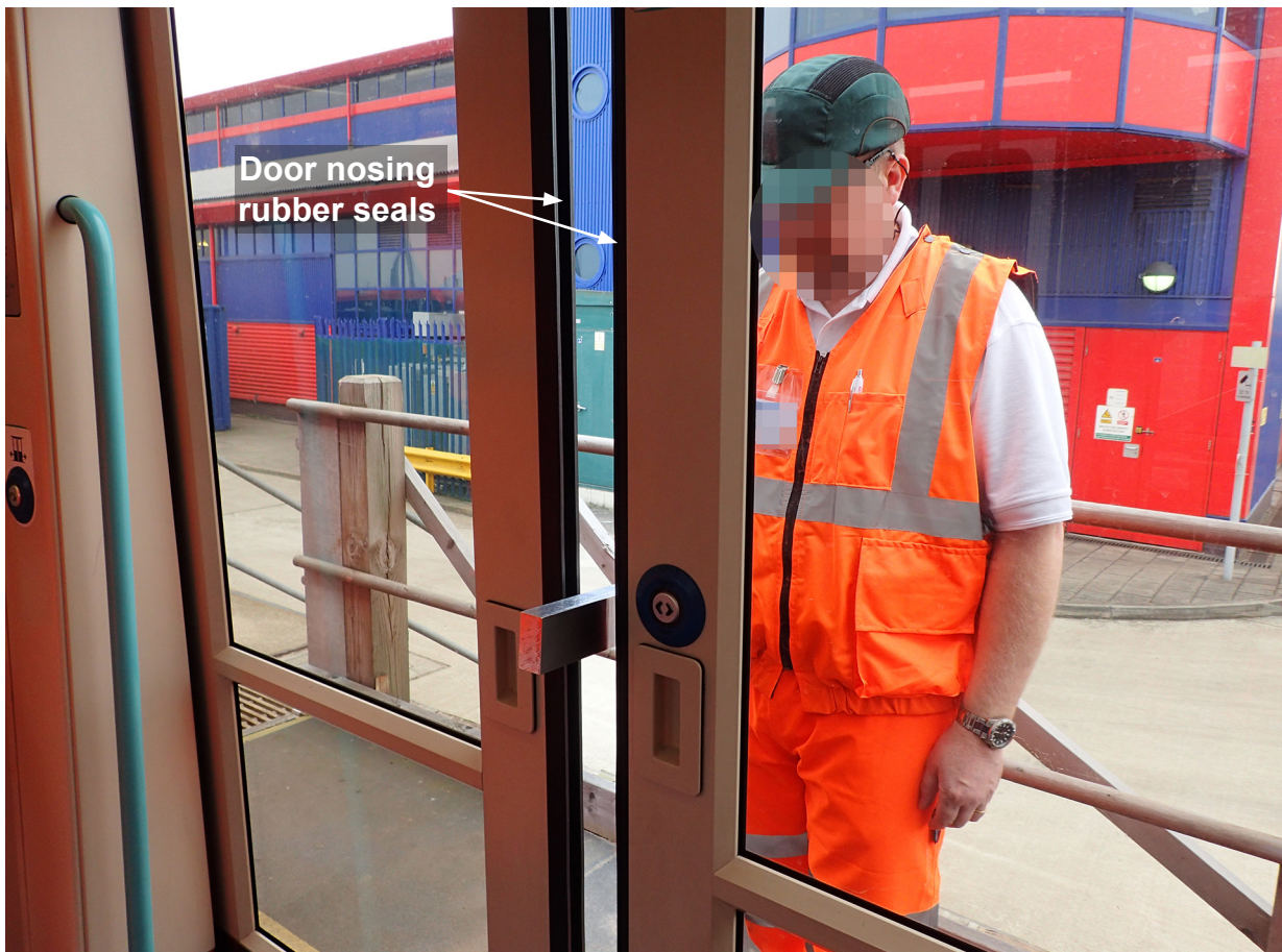
Figure 8: Testing of the door system
