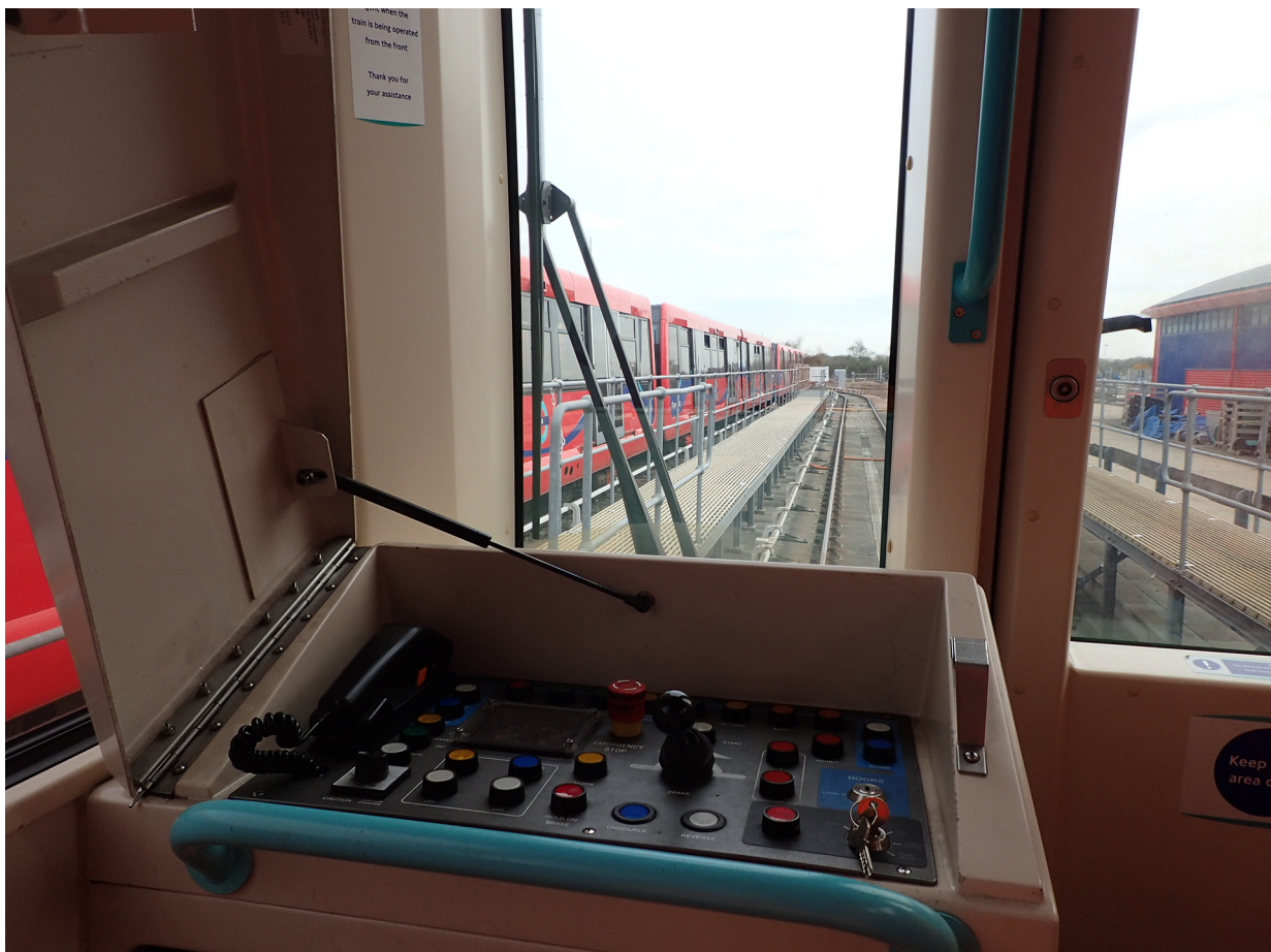
Figure 5: Location of EDP (with cover lifted) at the front of a DLR car
