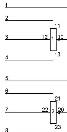
Fig. 1 Two-deck potentiometer
