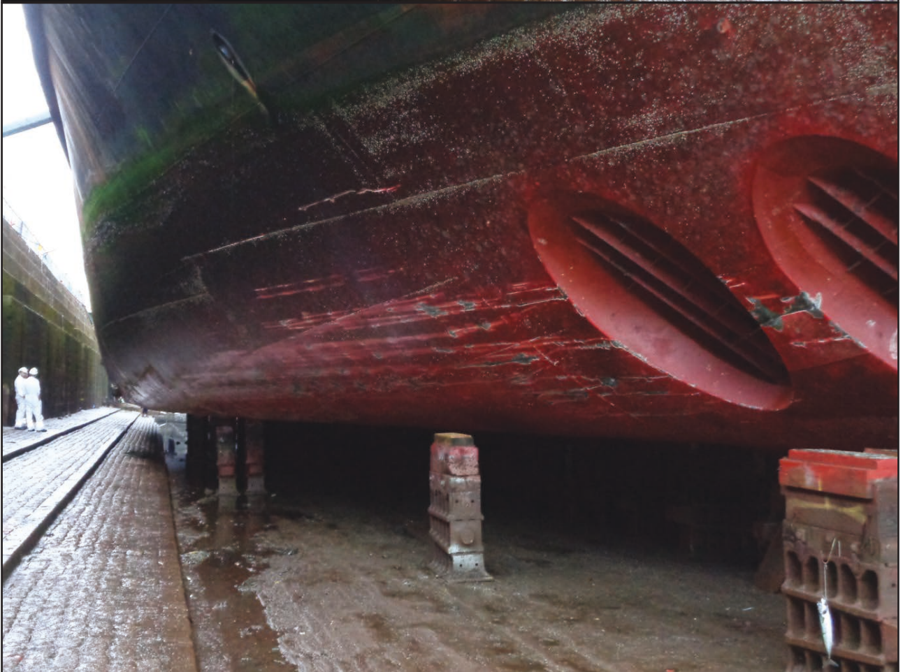
Figure 10: Damage to starboard bilge keel and hull bottom
