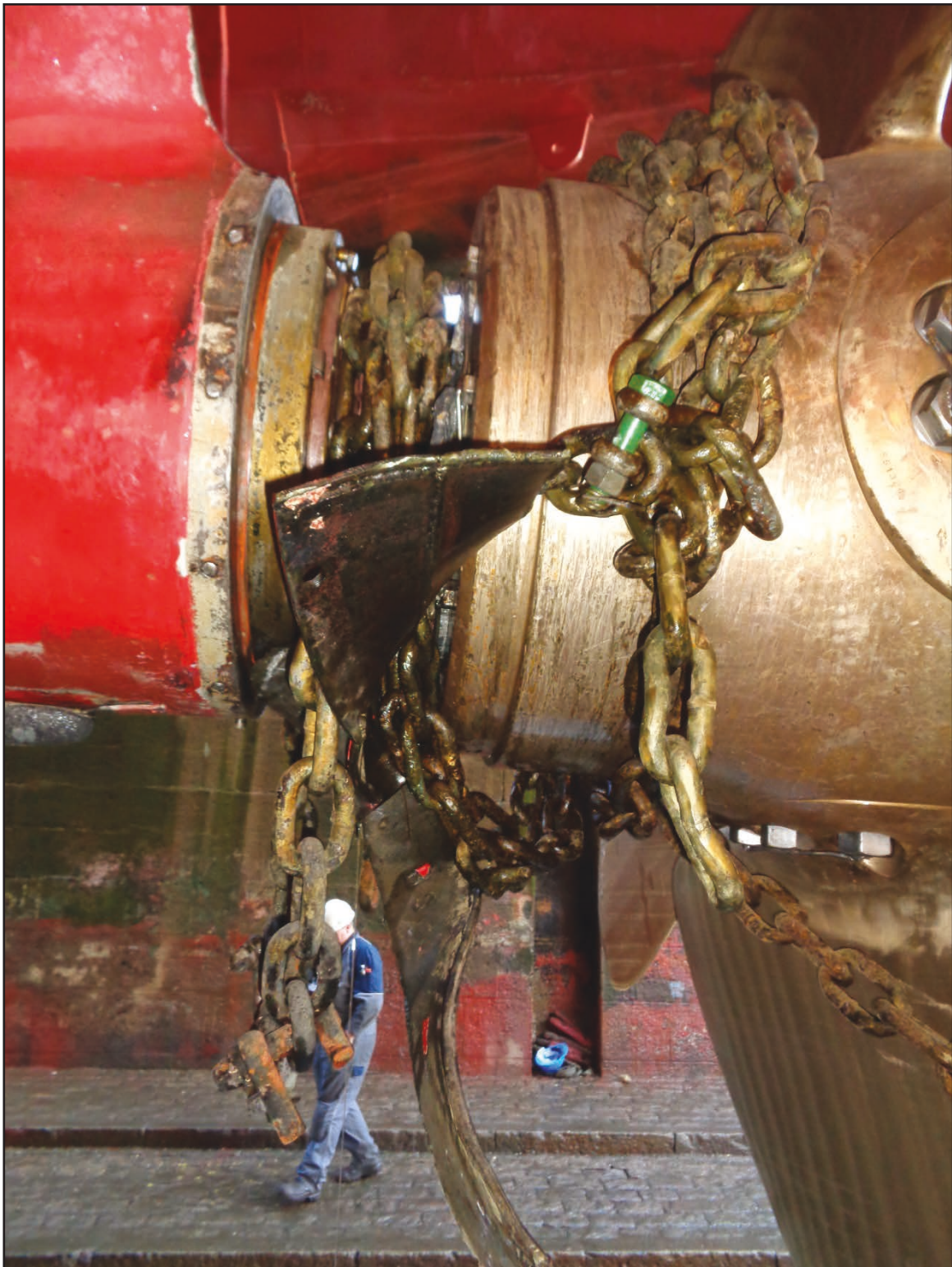
Figure 11: Mooring chain around starboard propeller
