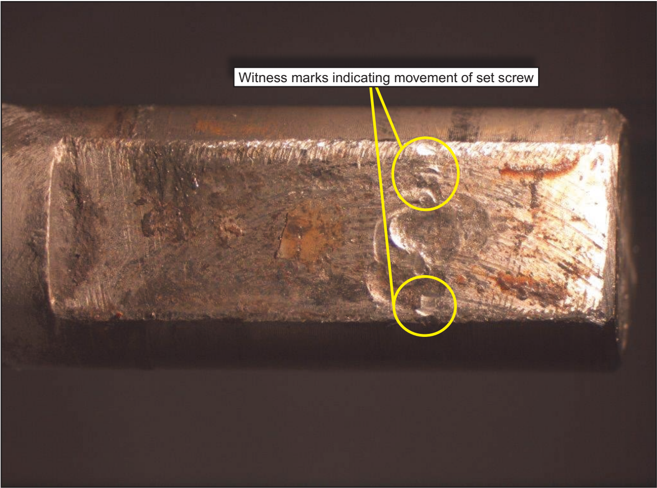
Figure 14: Marks on stepper motor shaft
