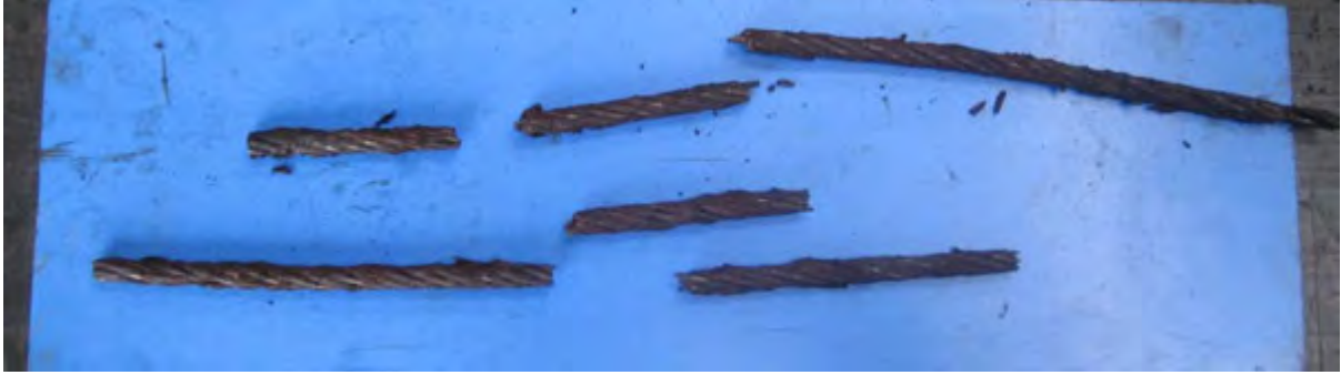
Figure 10.23: Tug side sample IWRC core - broken through in five places (6 pieces) over 1 m length.
