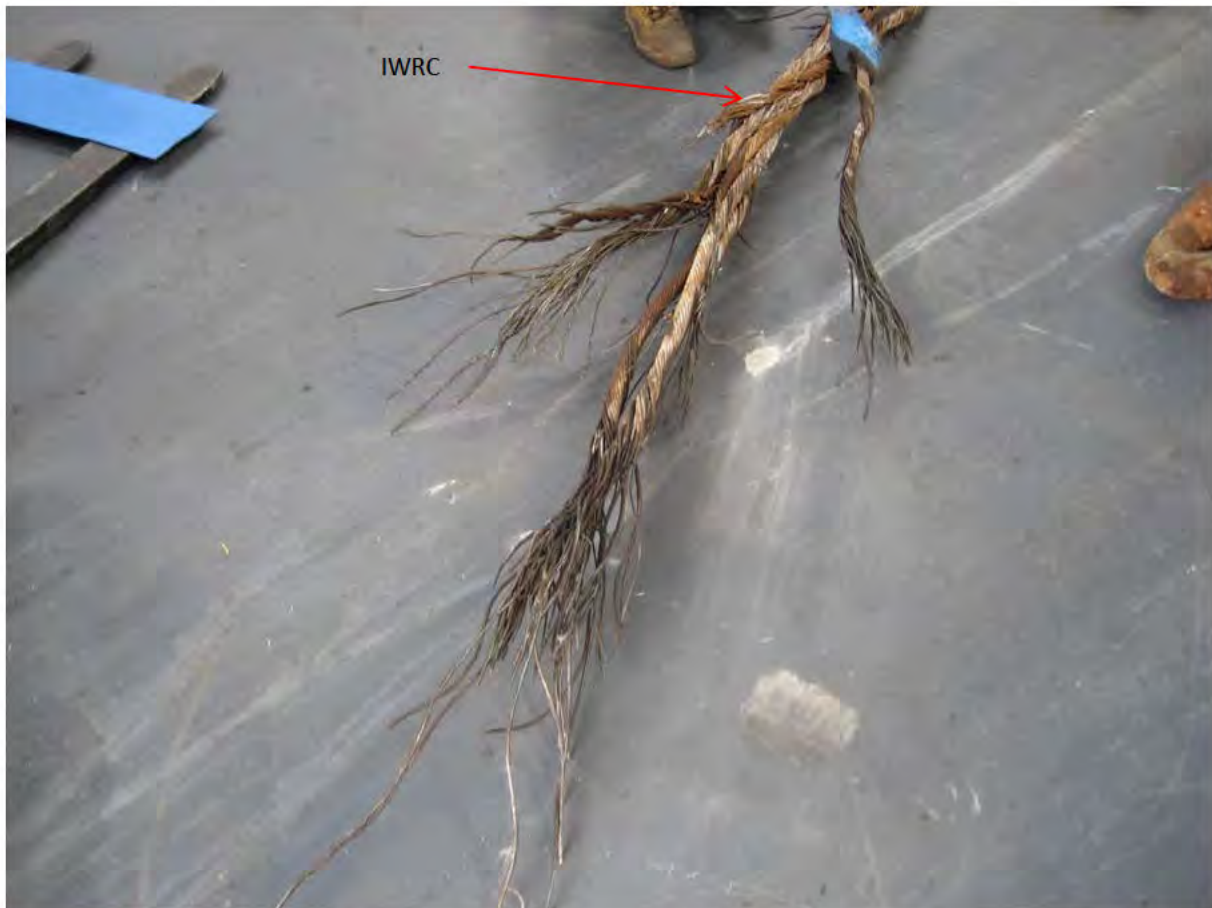
Figure 5.6: Failure of IWRC and five strands over a distance 18.0 - 19.2 m from the cut end on tug side sample.
