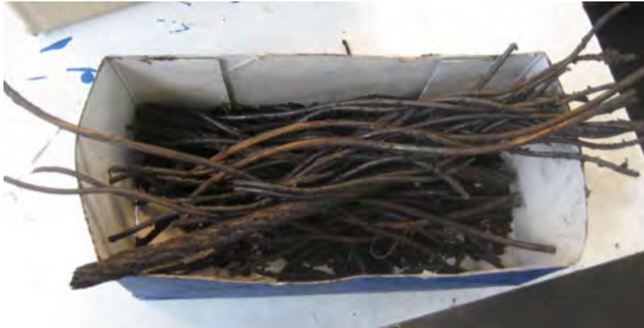
Figure 9.10: Broken wires found in preparation of Bridle sample terminations - mostly IWRC wires.
