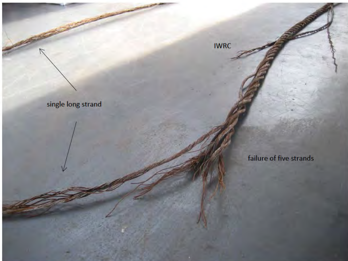
Figure 5.14: General view on main wire rope failure (rig sample).
