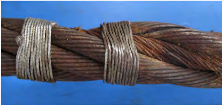
Figure 5.5: Seizing wire on wire rope measured at 12.96 m from cut end on tug side sample.
