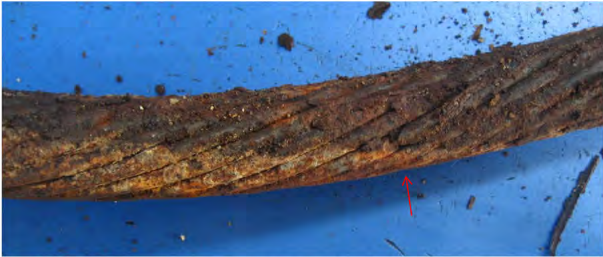
Figure 10.41: Bridle sample main strand as removed from the sample. The upper (darker coloured section) would have been towards the inside (IWRC), whilst the lighter section was on the outside of the wire rope. The intersection of these two areas is the valley position between the strands. Note the wire break at this interface (arrowed).
