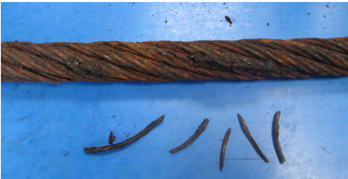
Figure 10.18: Tug side sample, general condition of IWRC. Five wires dropped out of the construction as the outer strands were removed. Some areas of good level, good nature lubricant, but on the whole the lubricant level was low and dry.
