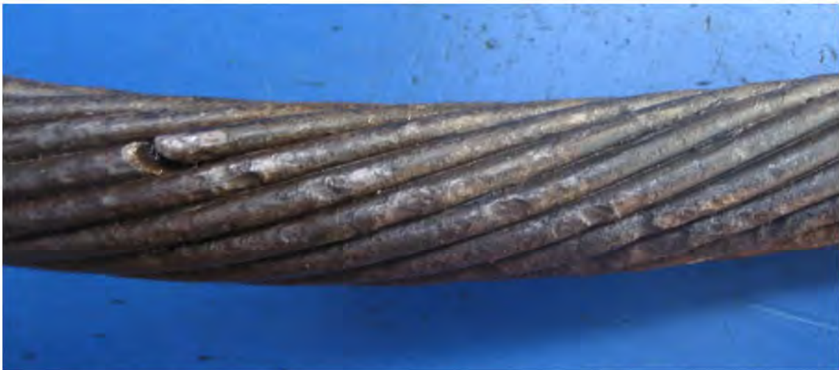
Figure 10.42: Bridle sample main strand after cleaning. Note the series of elliptical wear patches along the valley position from which wire breaks have/will initiate.
