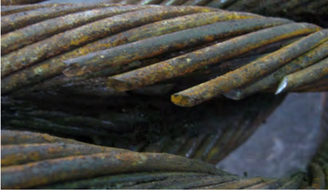
Figure 9.12: Bridle sample after testing, detailed view on wire failures (old - rusty ends, new - shiny).
