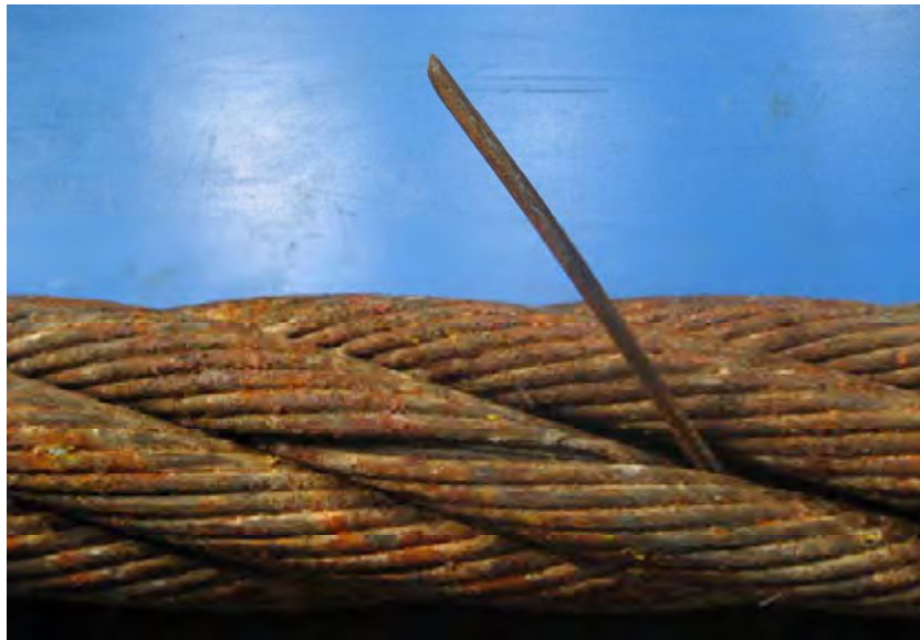
Figure 5.7: Outer strand wire break (valley) measured at 1.4 m from cut end on tug side sample.
