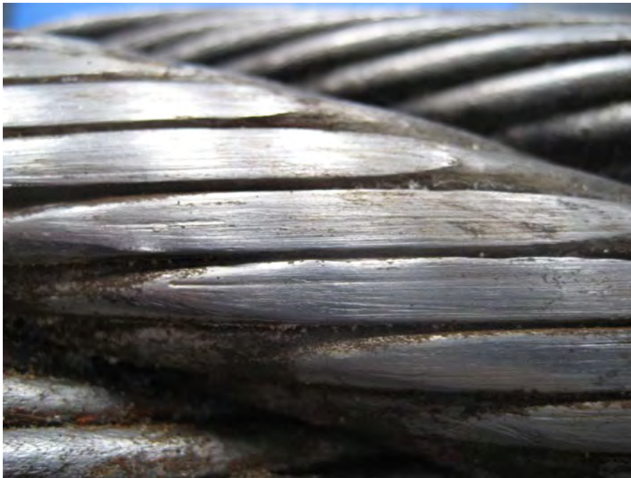
Figure 5.11: Significant abrasion on the surface of the outer wires 2.0 m from cut end of rig side sample.
