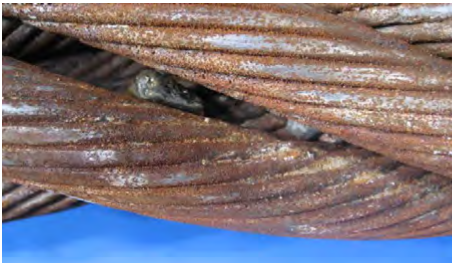
Figure 5.12: Small pieces of stone noted trapped in the wire rope at 5.6 m from cut end of rig sample.
