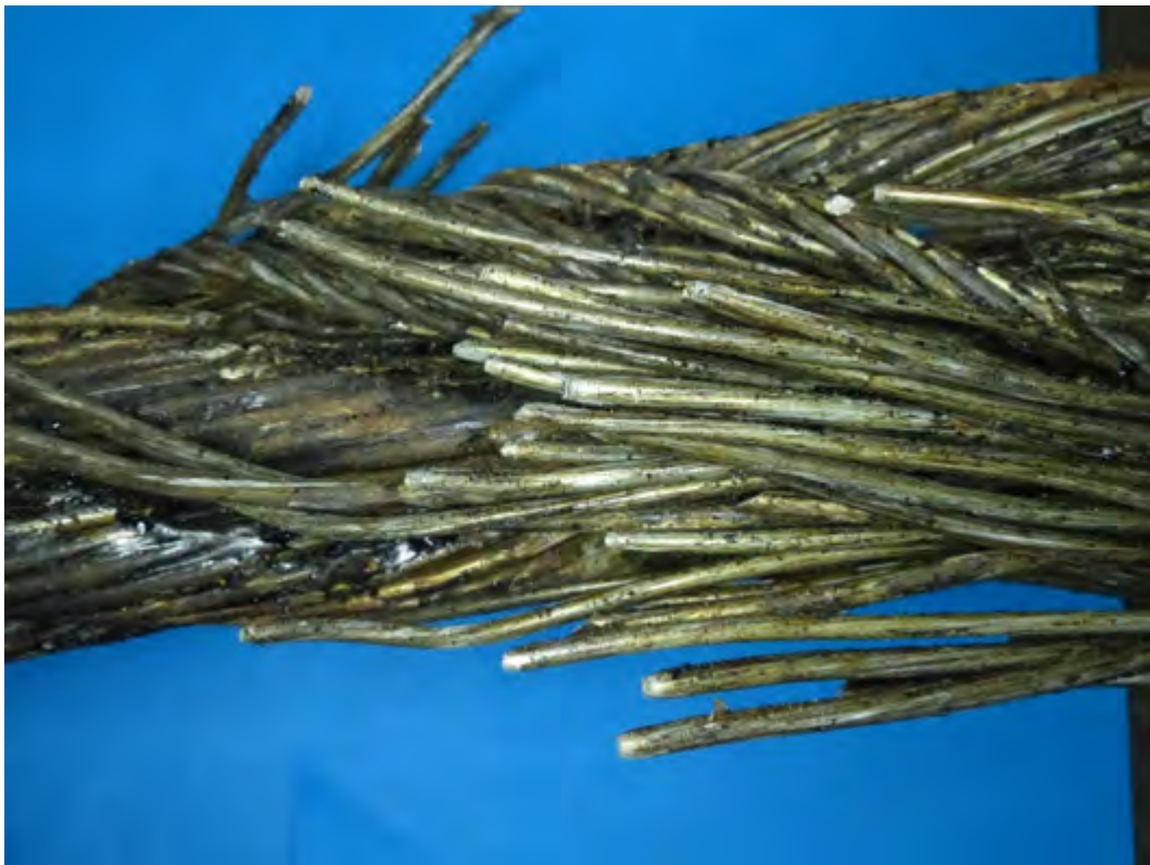
Figure 9.5: Drum sample detailed view on failure region.
