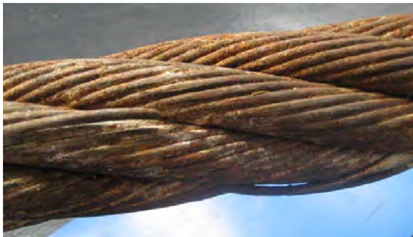
Figure 5.8: Two of six outer strand wire breaks measured at 2.0 m from cut end on tug side sample.
