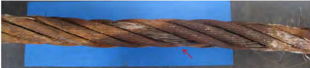
Figure 5.3: Strand failure noted at 10.6 m from cut end on tug side sample (started at 10.2 m).
