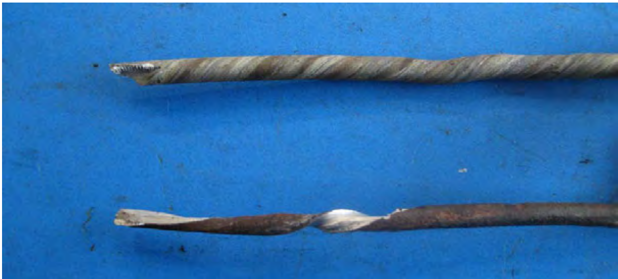
Figure 14.6: Appearance of wire failures in torsion tests on wires from the bridle sample. (Bottom OS1 OW3 (3 turns/100d w ), top OS1 CW (30 turns/100d w )).
