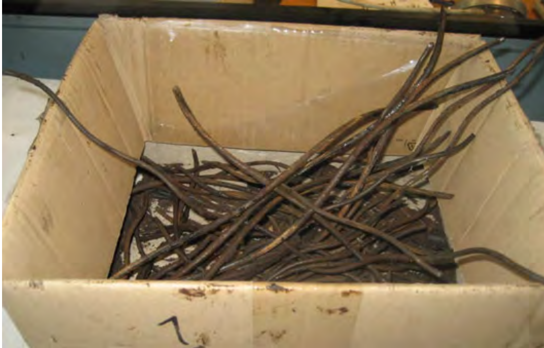
Figure 9.6: Tug side sample - broken wires found in preparation of sample terminations. (Mostly IWRC wires, but also some outer strand outer wires).
