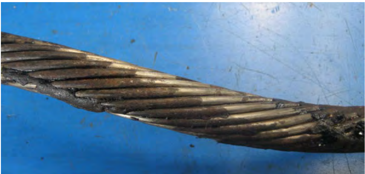
Figure 10.4: Drum sample outer strand partially cleaned to show the difference in residual galvanising levels for sections on the inside and outside of the wire rope.
