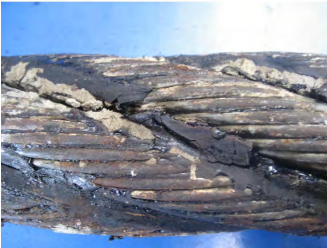
Figure 10.2: Detailed view on the drum sample showing an area of corrosion. Note also the 'mud deposits' and the good level of lubricant in the valleys.
