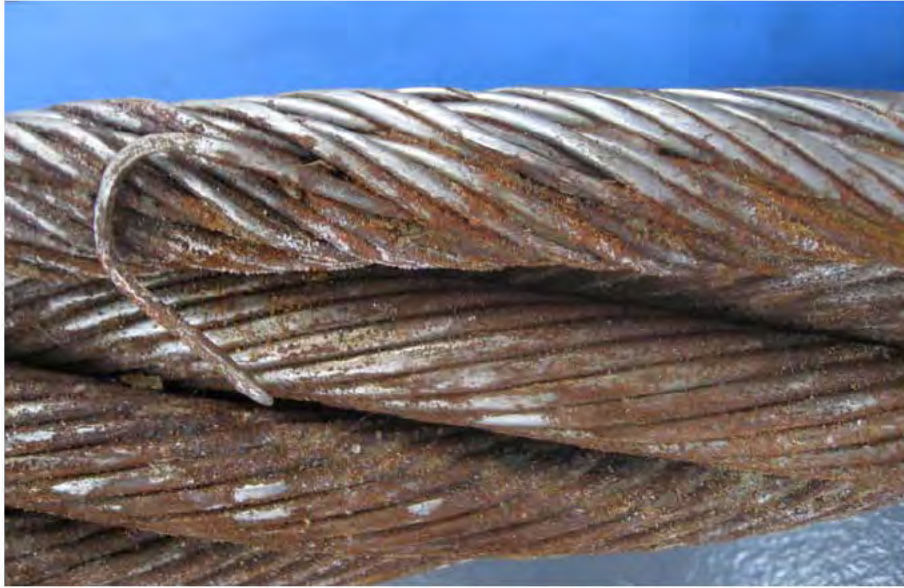
Figure 5.13: Abrasion (and wire breaks) noted on the displaced IWRC at 7.2 m from cut end of rig sample.
