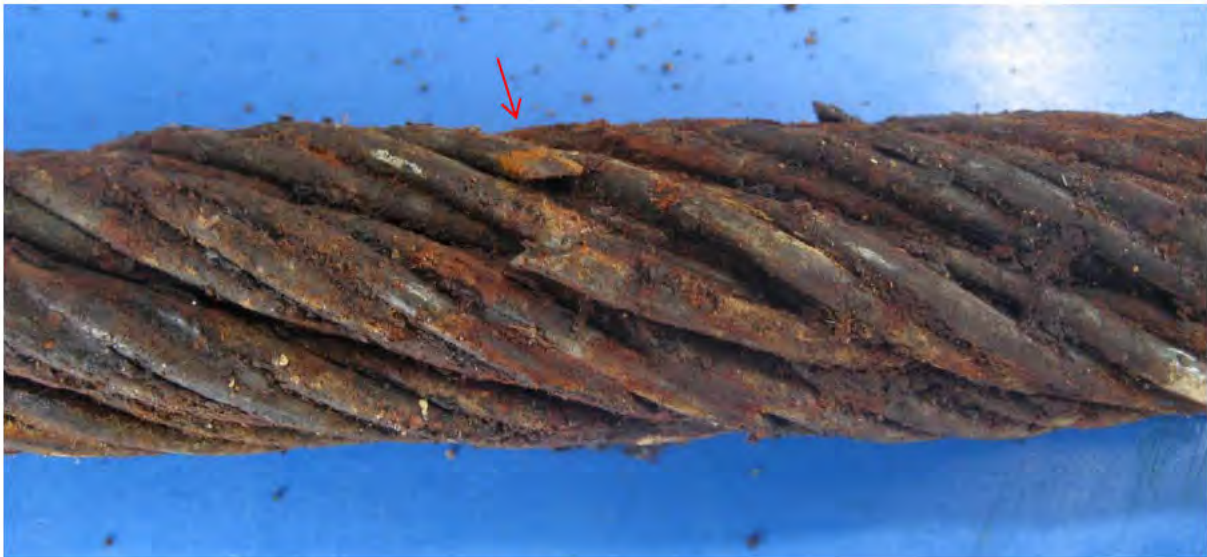
Figure 10.20: Wire breaks found in tug side sample IWRC outer strands (recent wire break arrowed).
