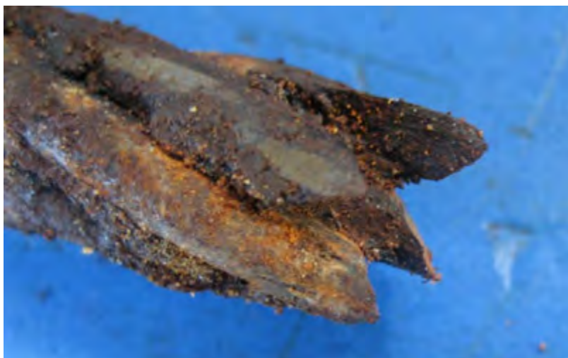
Figure 10.37: Bridle sample IWRC core showing typical shear type wire failures.
