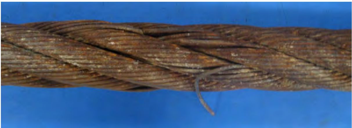
Figure 8.2: Group of at least eight wire breaks noted at 15.2 m on the bridle sample.
