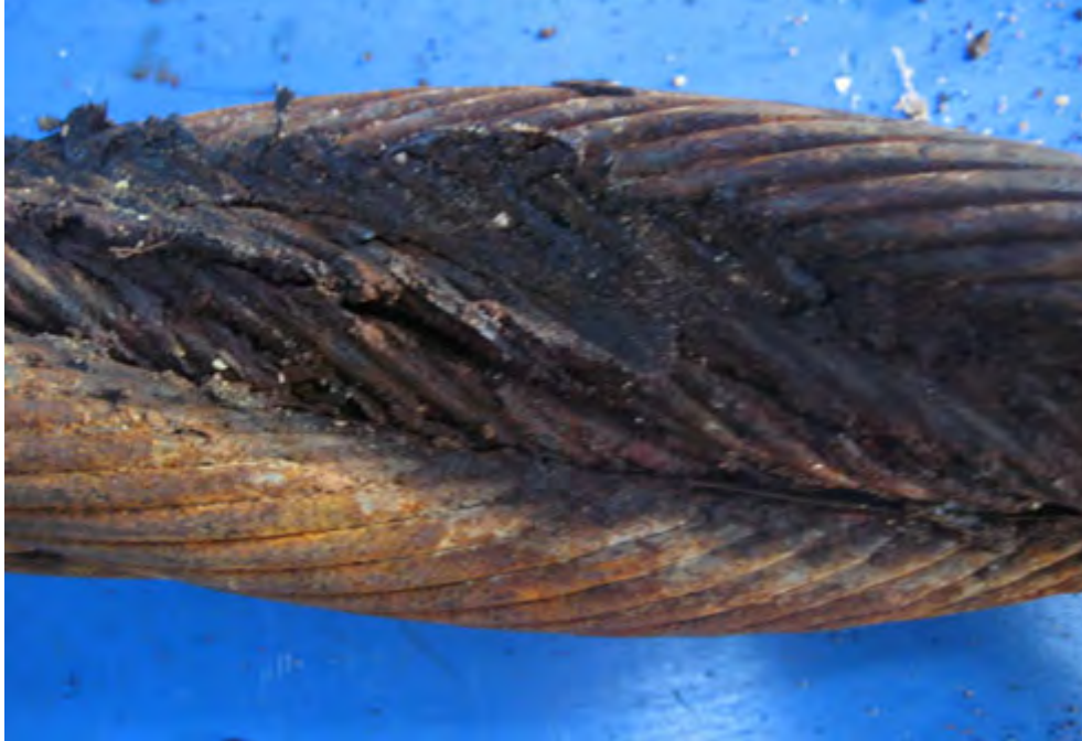
Figure 10.32: Bridle sample with two outer strands removed - area of good lubrication on IWRC.
