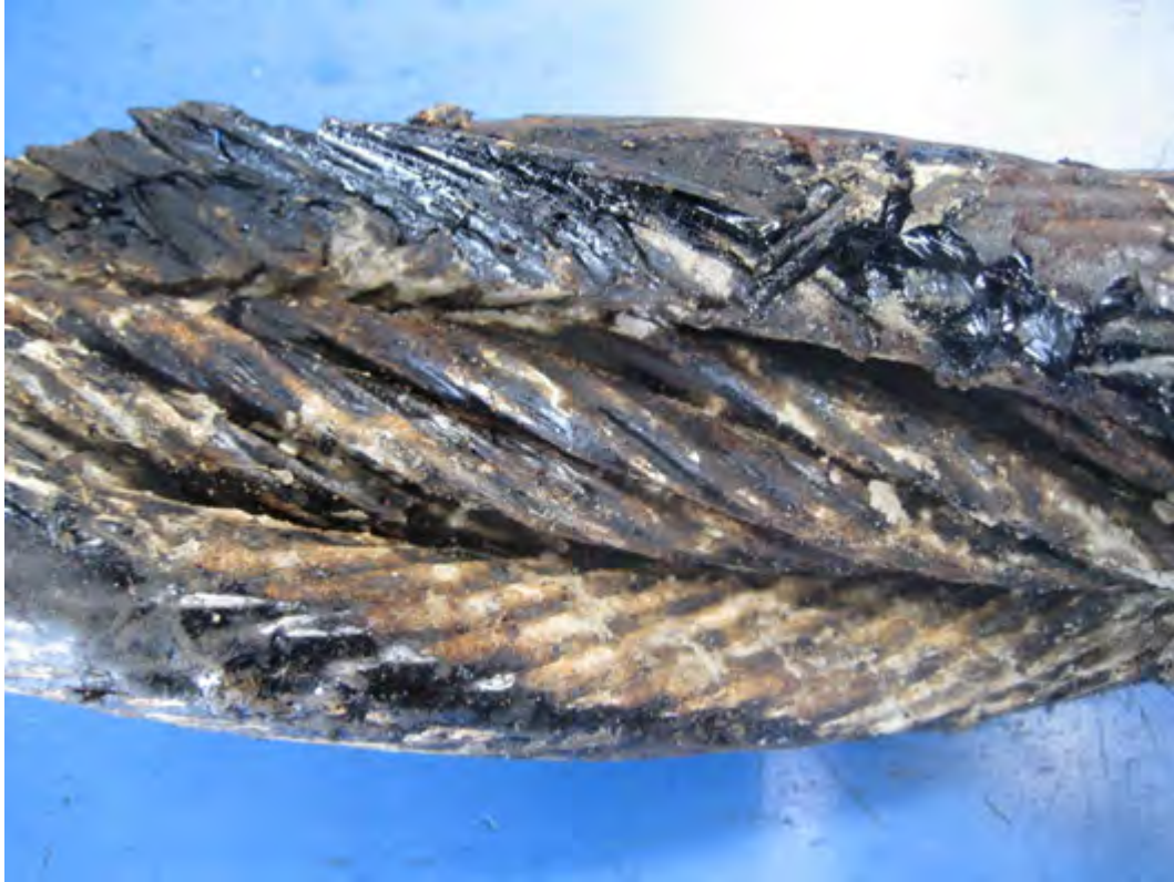
Figure 10.3: Drum sample with two outer strands removed to show the condition of the IWRC - the lubricant level is very low. Note also the light corrosion on the outer strand (top right) and the glassy bitumous lubricant in the valley positions (of the outer strands).
