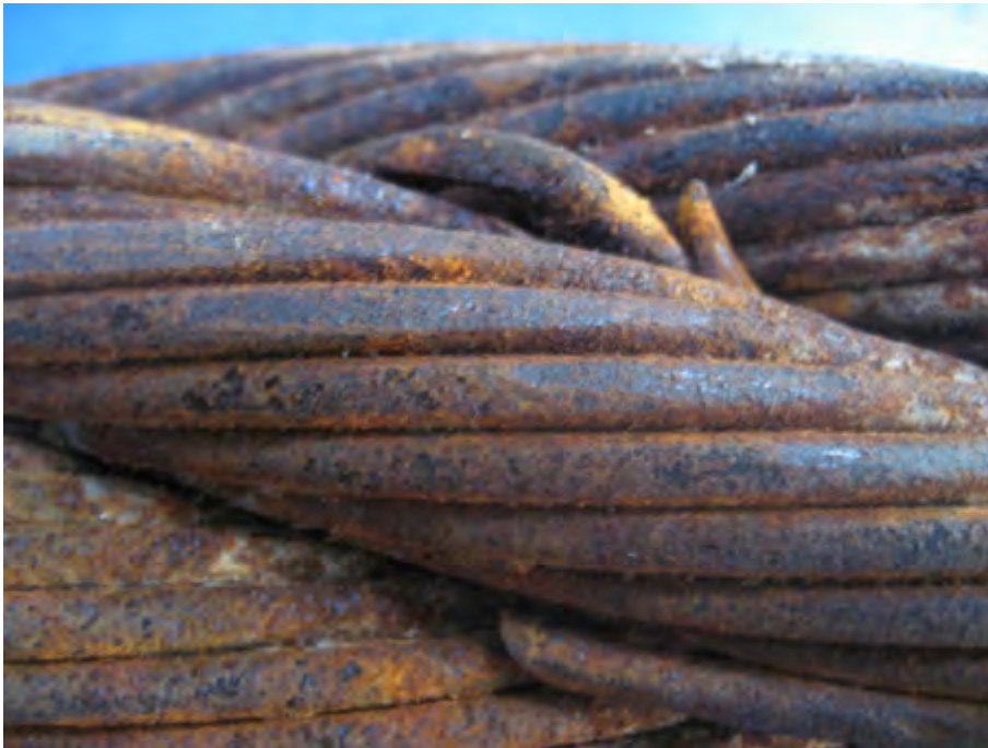
Figure 10.31: Detailed view on bridle sample - note no visible galvanising and a uniform covering of corrosion causing roughening of the surface of the wires.
