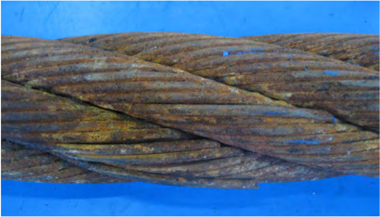
Figure 8.3: Group of at least six wire breaks noted at 16.5 m on the bridle sample (the blue paint is from the shipping container).
