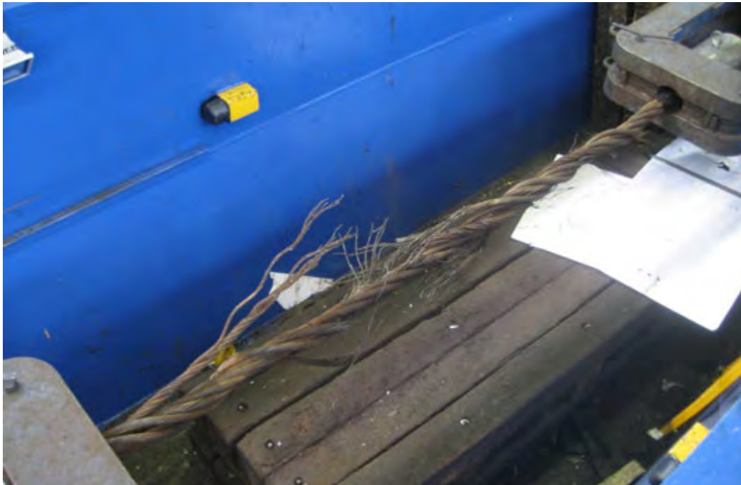
Figure 9.7: Tug side sample after testing, failure mid-length.
