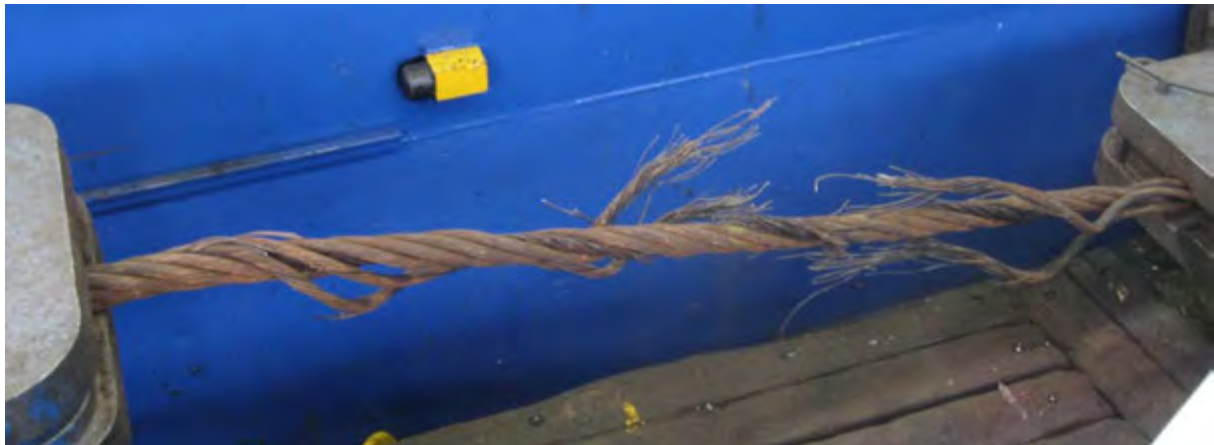
Figure 9.11: Bridle sample after testing, failure mid-length.
