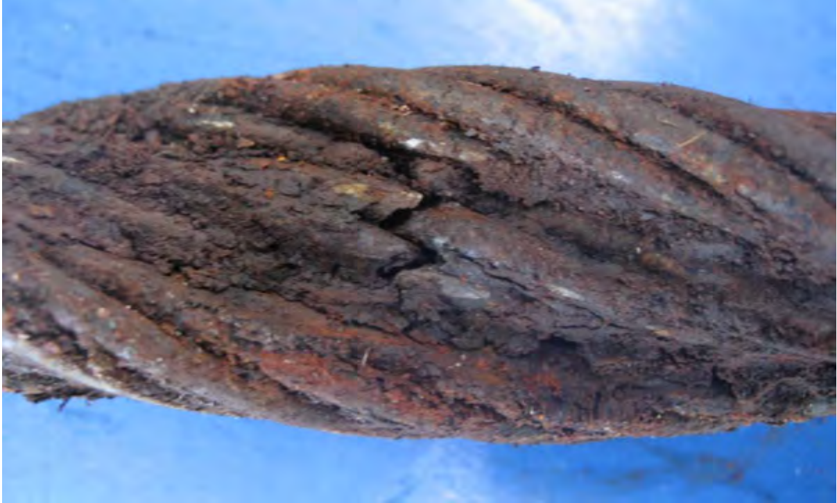
Figure 10.21: Tug side sample, IWRC with two strands removed to show core. Core strand broken through. Good level of lubricant.
