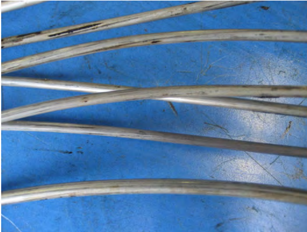
Figure 10.7: Drum sample outer strand - third layer of wires and core wire (bottom).
