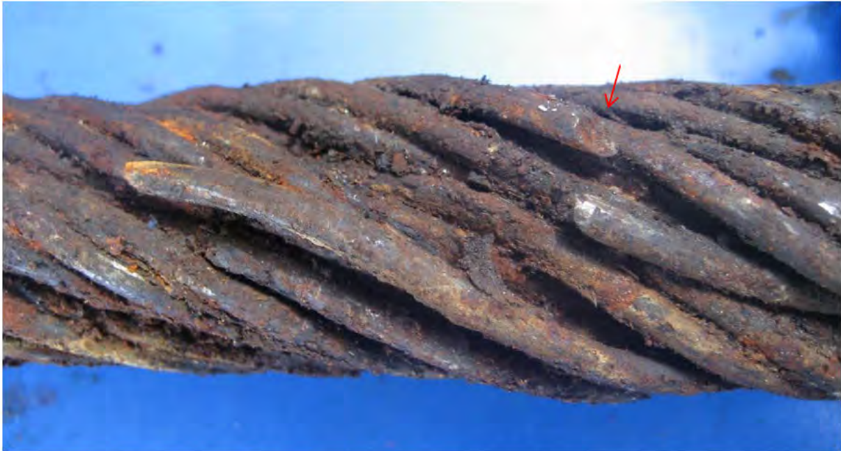
Figure 10.19: Wire breaks found in tug side sample IWRC outer strands (existing wire break arrowed).
