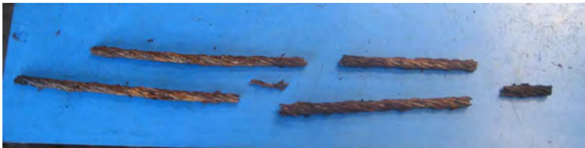
Figure 10.36: Bridle sample IWRC with three outer strands removed to show the core (all core strand wires broken).
