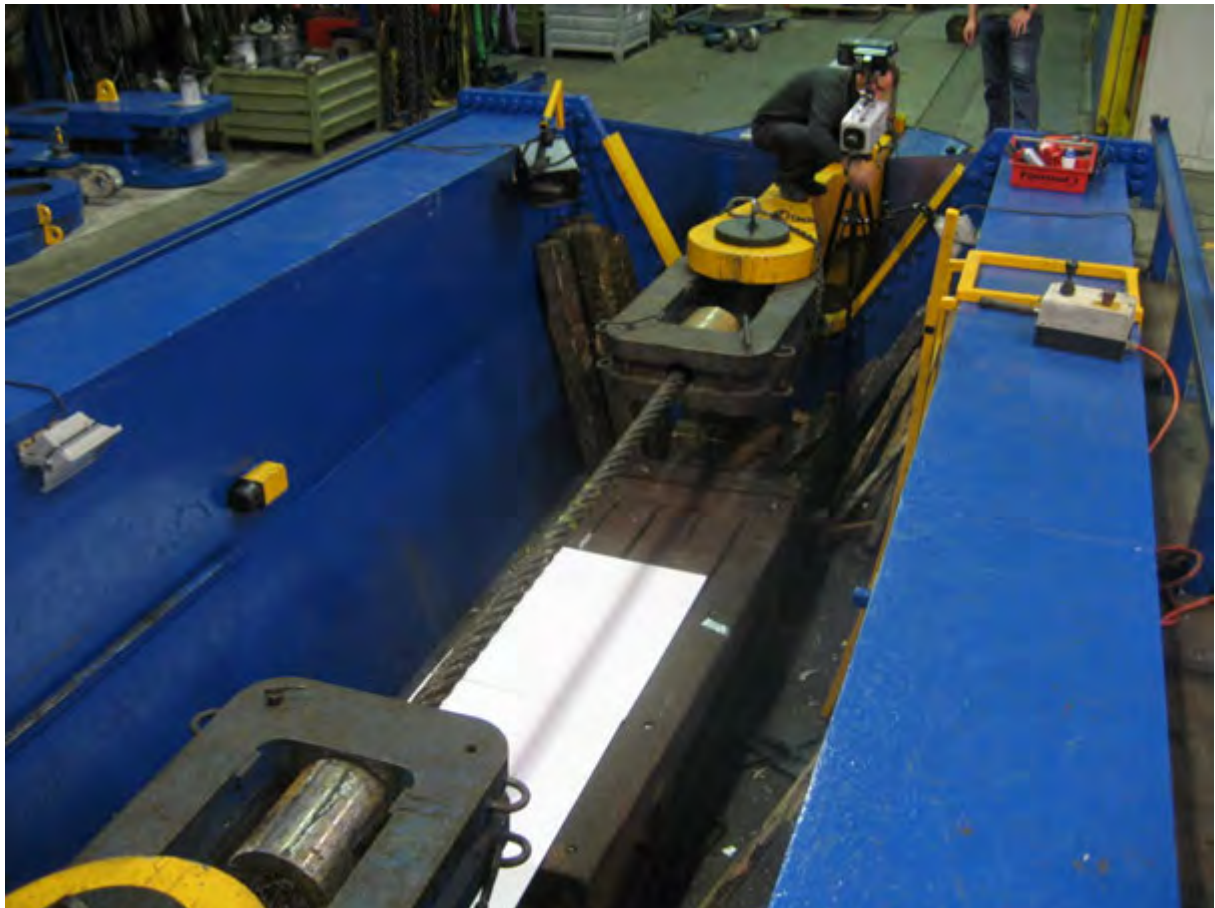
Figure 9.1: Wire rope sample ready for testing in Mennens' 1,400 tonne tensile testing machine.
