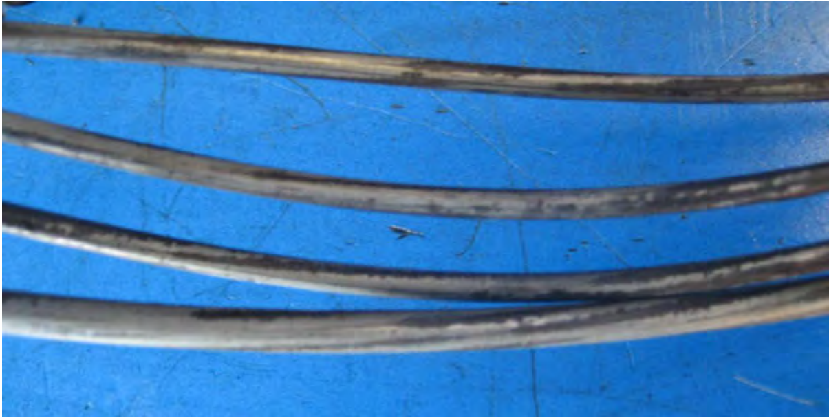
Figure 10.45: Bridle sample main strand (some of) the third layer of wires and core wire (bottom).
