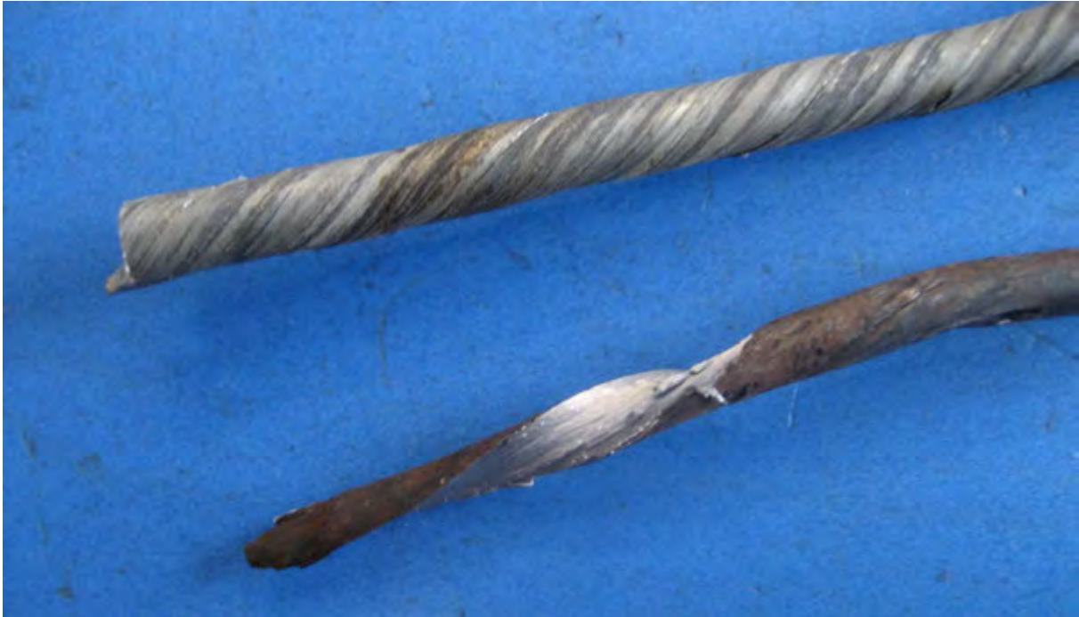
Figure 14.4: Appearance of wire failures in torsion tests on wires from the tug side sample. (Bottom OS OW1 (3 turns/100d w ), top OS CW (27 turns/100d w )).
