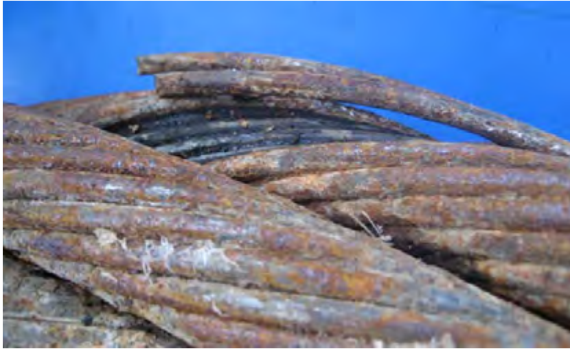
Figure 5.9: Two outer strand wire breaks measured at 5.6 m from cut end on tug side sample.
