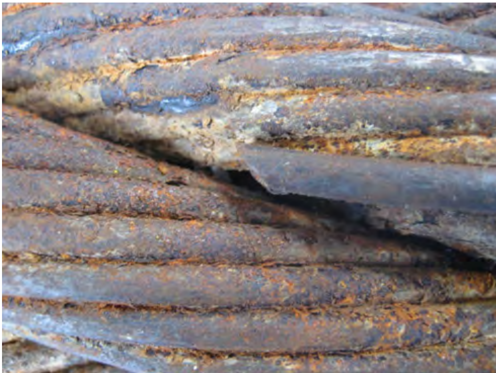
Figure 10.16: Detailed view on single wire break noted in valley position on tug side sample.
