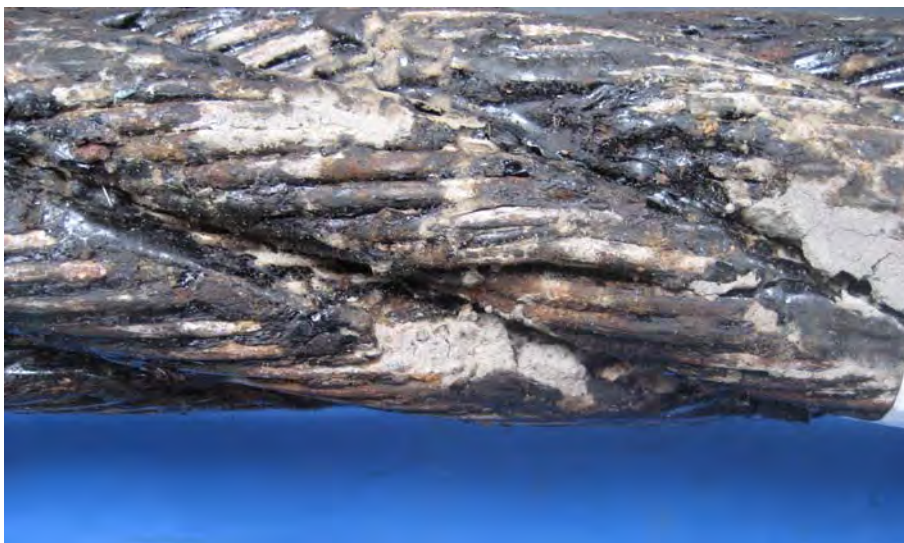
Figure 5.2: Area of crushing damage found on the drum sample (mid-length).
