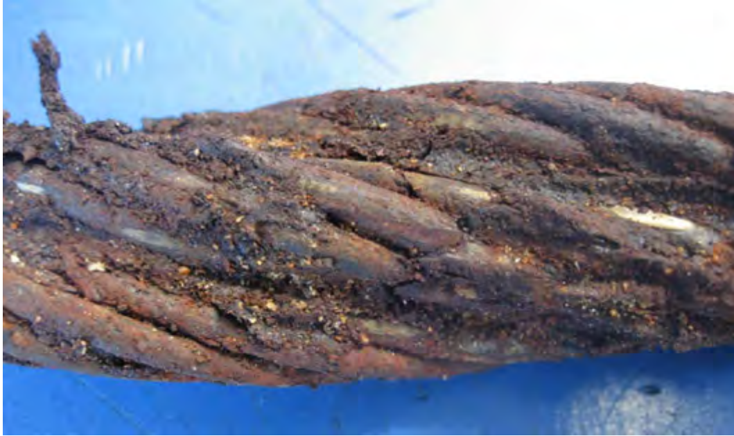
Figure 10.35: Bridle sample IWRC with three outer strands removed to show the core (all core strand wires broken).
