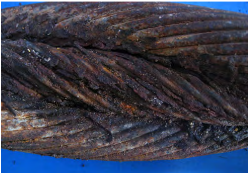
Figure 10.33: Bridle sample with two outer strands removed - area of low lubrication on IWRC.
