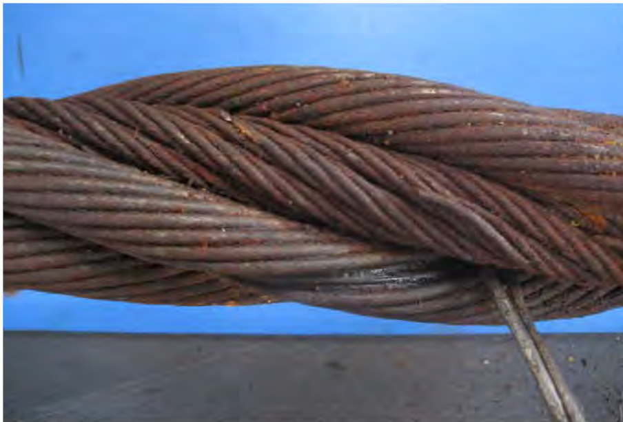
Figure 5.4: IWRC displaced from the centre of the wire rope at 12.5 m from cut end on tug side sample.
