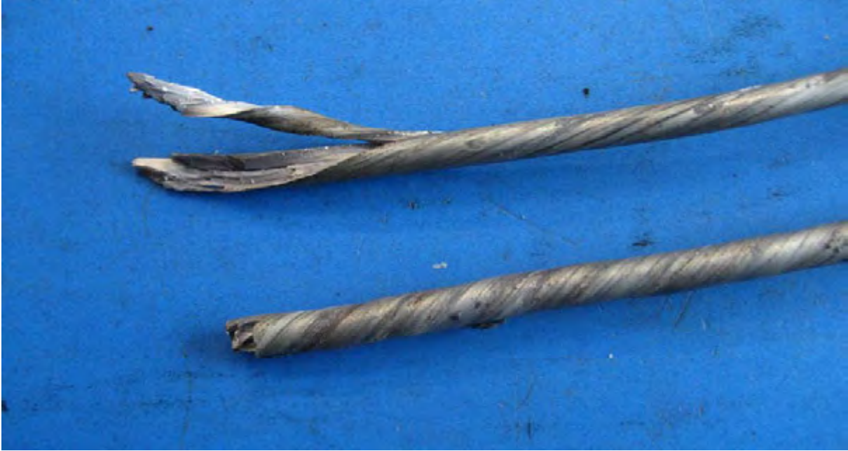
Figure 14.2: Appearance of wire failures in torsion tests on wires from the drum sample. (Top OS OW1 (7 turns/100d w ), bottom OS CW (27 turns/100d w )).
