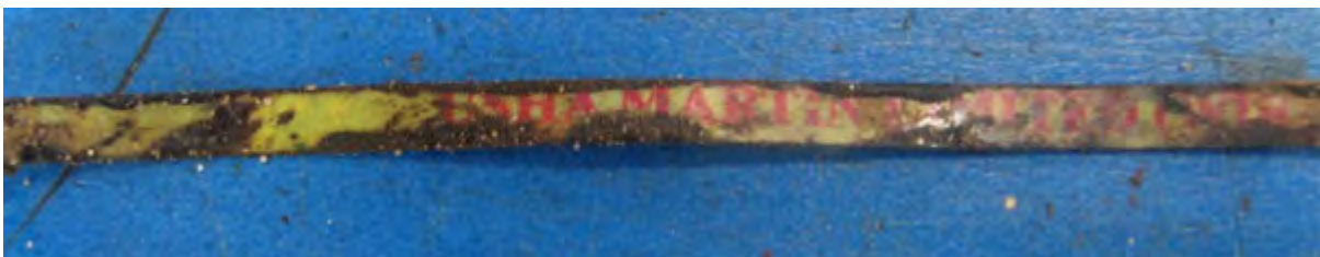
Figure 10.8: Manufacturers' identification tape found under the outer strands and on the IWRC (Drum sample).
