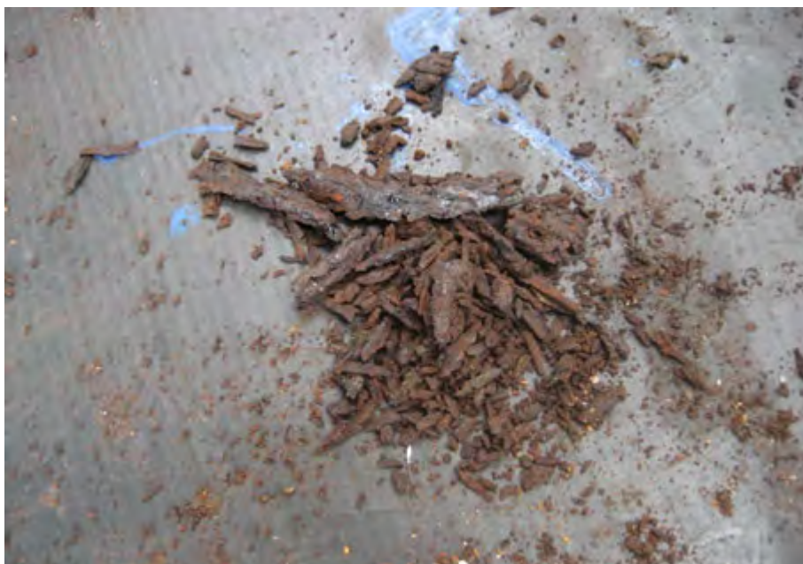
Figure 10.22: Tug side sample, dry lubricant which dropped out of the wire rope.
