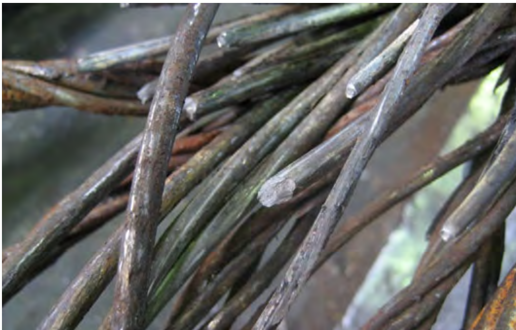
Figure 9.9: Tug side sample after testing, detailed view on wire failures.
