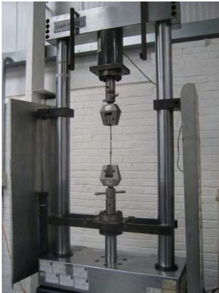
Figure 12.1: Tensile testing of wire in 250 kN tensile testing machine.
