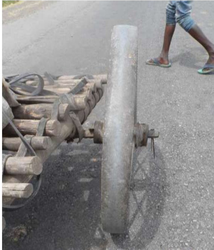
Figure A.19: Close-up of steel wheel on a donkey cart showing curved profile
