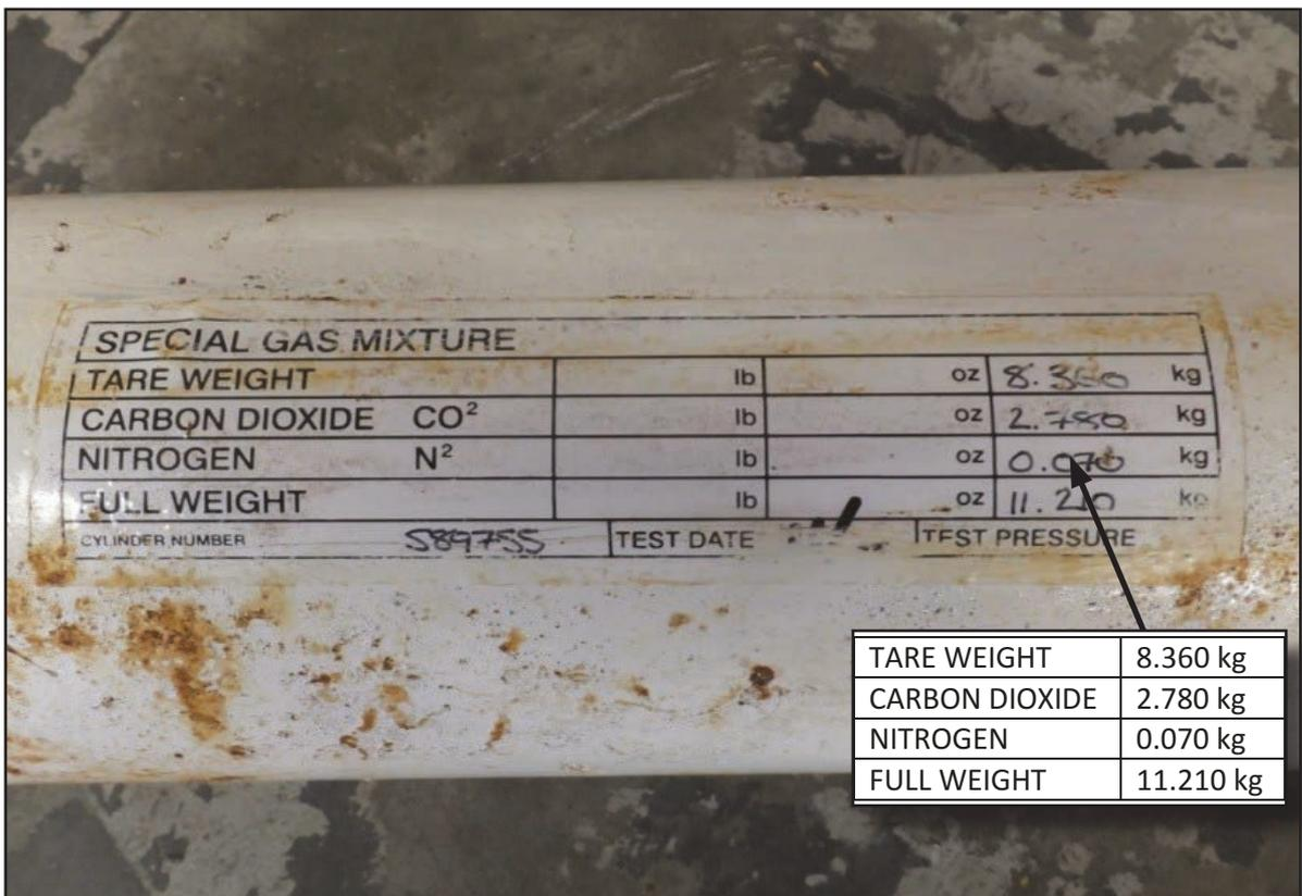
Figure 9: Recalled CO<sub>2</sub> cylinder of a similar type to that of *Louisa's* cylinder
