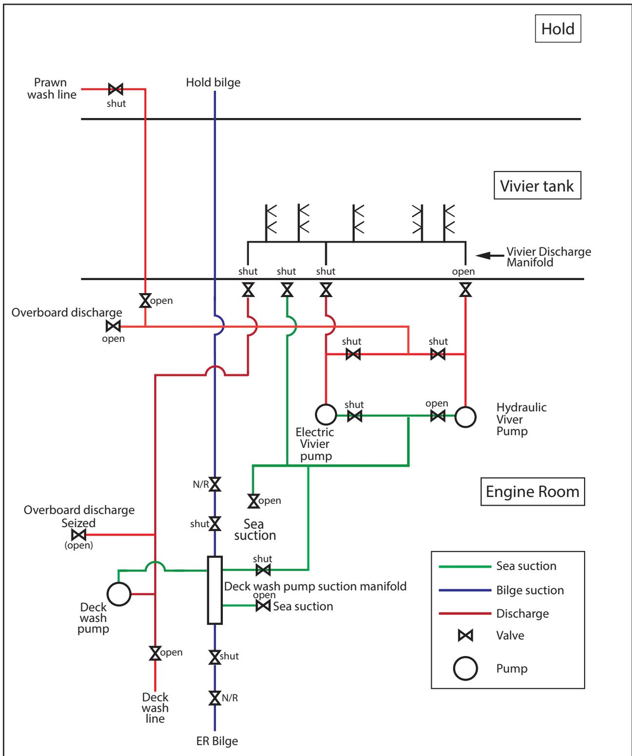
**Figure 6:** System drawing (valves as found)
