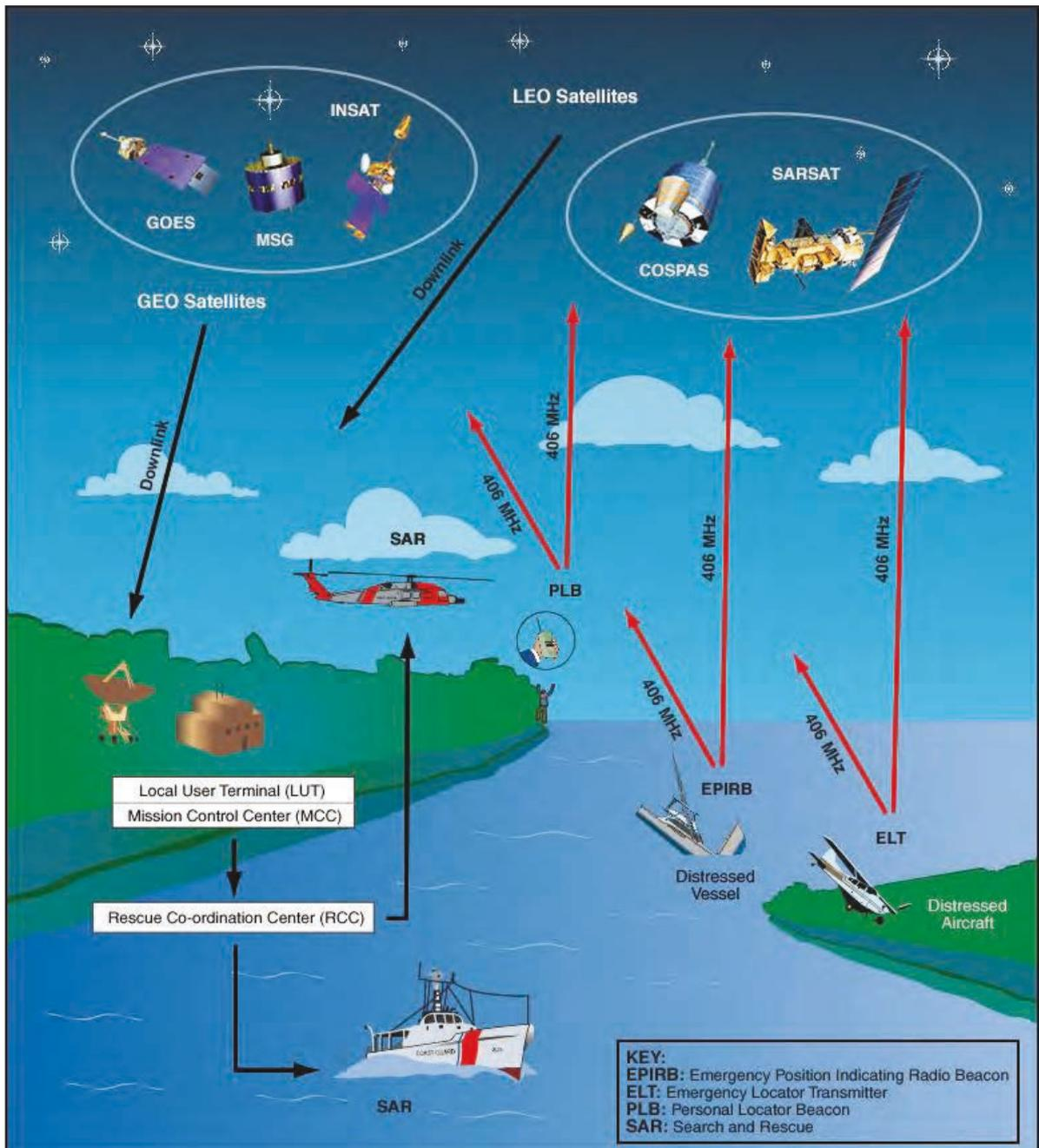
Figure 13: Cospas-Sarsat system diagram
