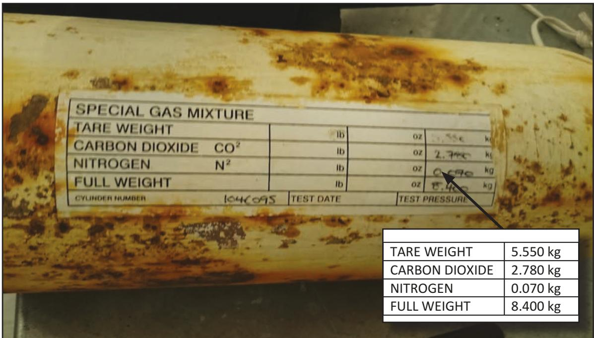
Figure 8: CO<sub>2</sub> cylinder as found
