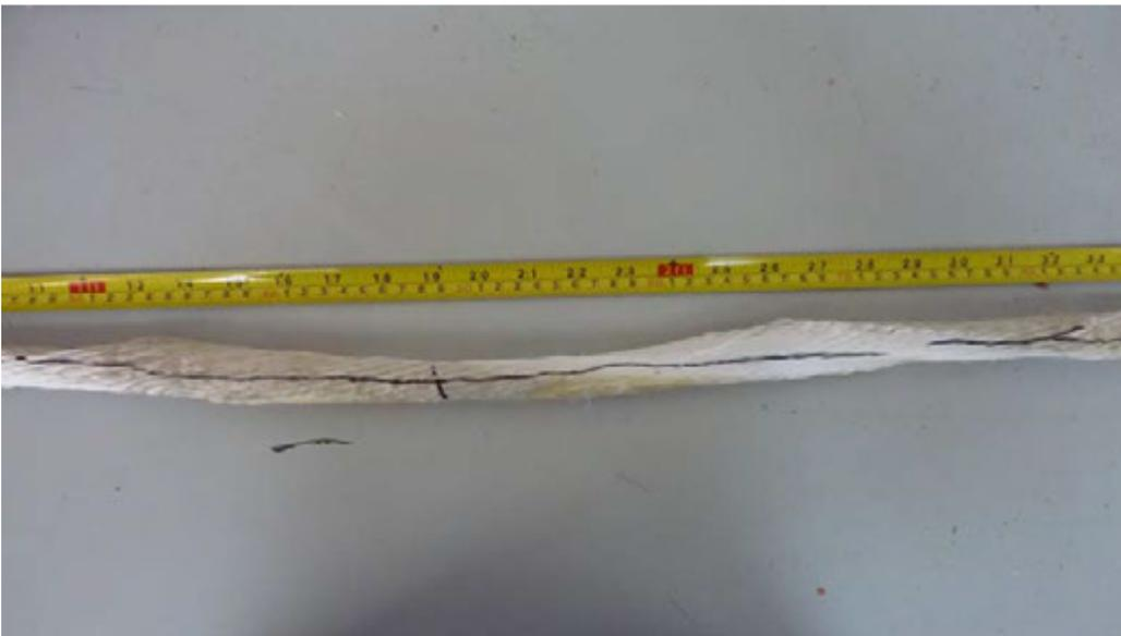
Figure 2.1 Strand removed from subrope to measure pitch
