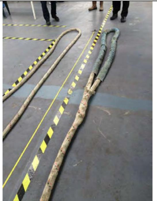
Figure 3.1.2 – Factory finished eye and splice
