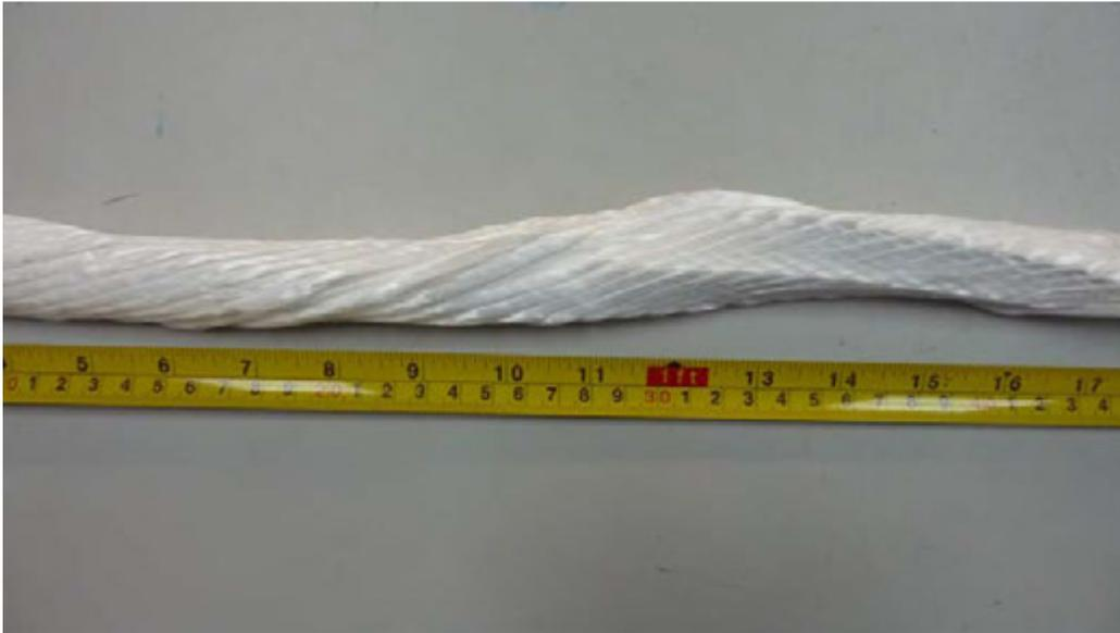
Figure 4.1.15: Sample 3, strand unlayed, very minor buckling outer layer rope yarns (cannot really see from this side of strand, see figure 4.1.19).
