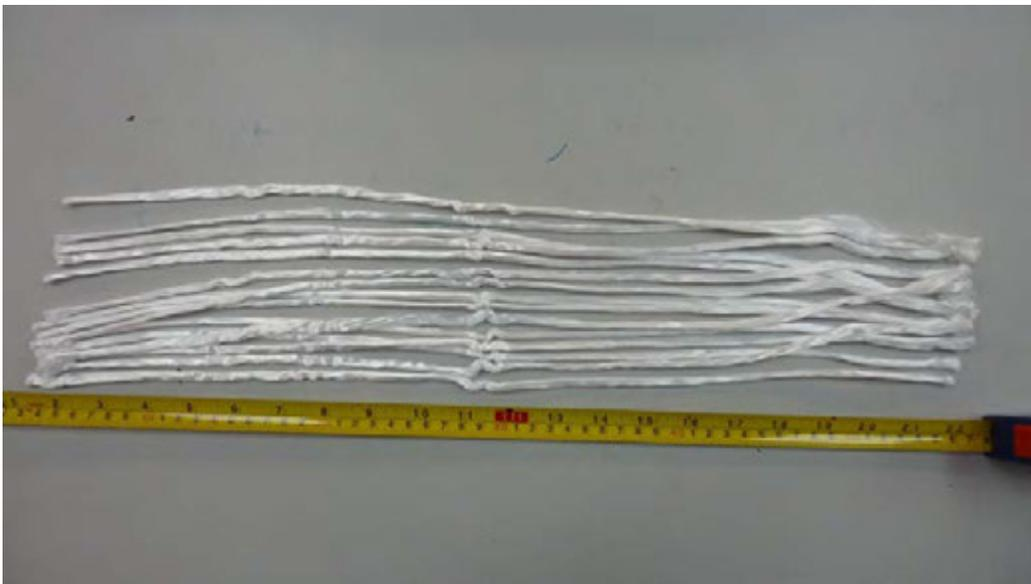
**Figure 4.1.10:** Sample 2, unlaidd strand to reveal inner rope yarns, most severely buckled.
