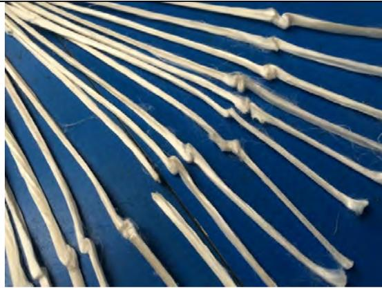
Figure 6.4 – Shore end – inner yarns - single yarn failure and partial failure failures
