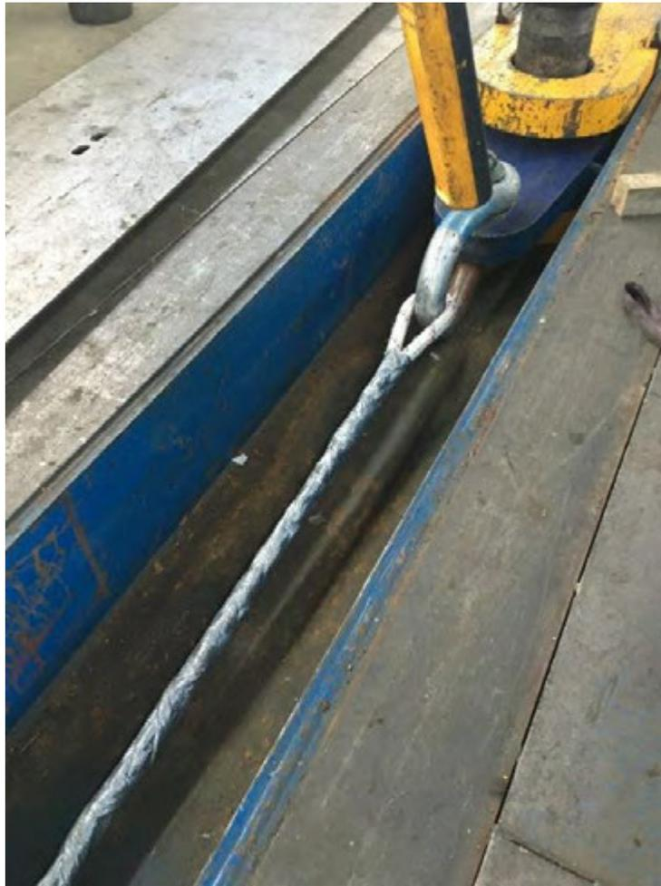
Figure 4.3.2: Rope sample 2 installed in test bed. Looking towards dead end.
