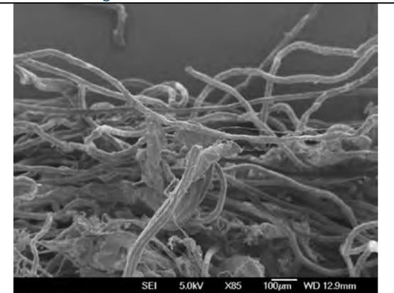
Figure 8.28 – close up of tensile failure end
