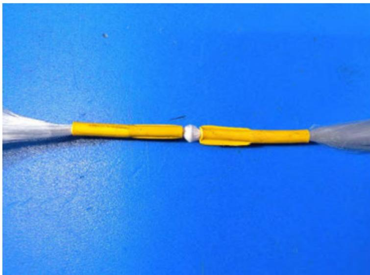
**Figure 3.4:** Image showing an unrestrained yarn bundle sample prior to break
