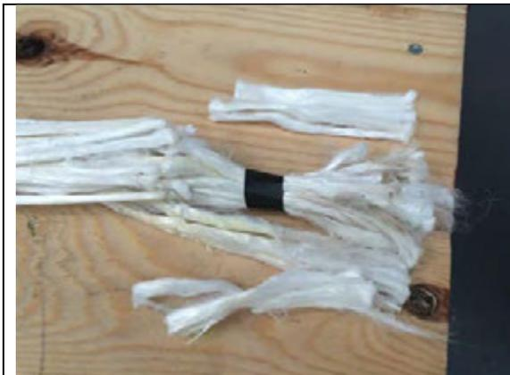
Figure 4.1.1 – Original Shore side sample – yarn failures
