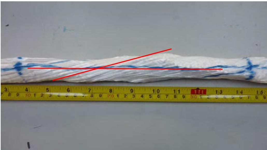
Figure 4.1.2: Sample 1, strand unlaidd, and showing only minor buckling to the outer layer yarns (cannot really see from this side of strand, see figure 4.1.5). Lay angle approx. 15 degrees and pitch 260mm.
