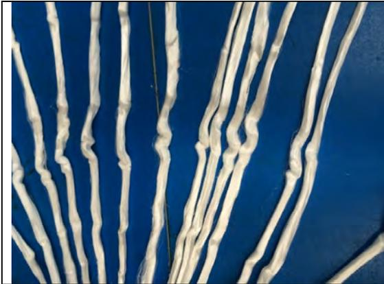
Figure 6.9 – Vessel Break end - Inner yarns with moderate kinks
