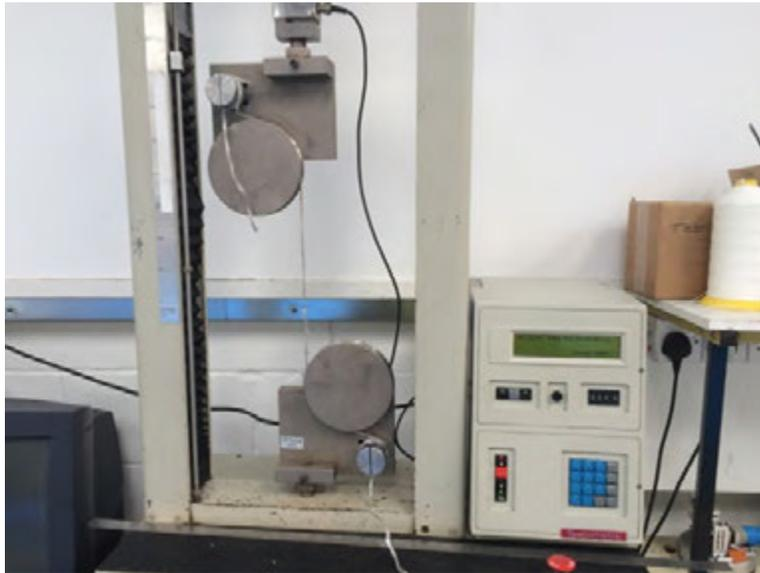
Figure 4.2.1.1: Testometric test machine
