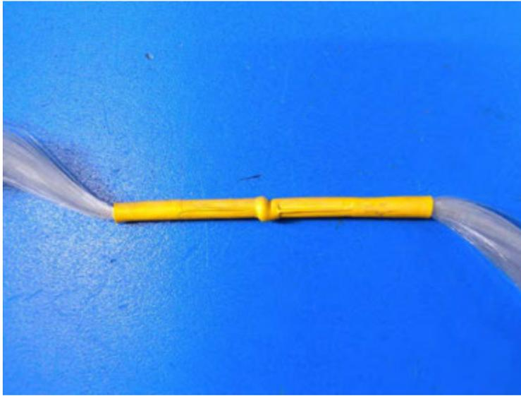
Figure 3.5: Image showing a restrained yarn bundle sample prior to break
