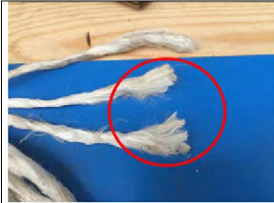
Figure 8.5 – Shore side possible kinkband failure
