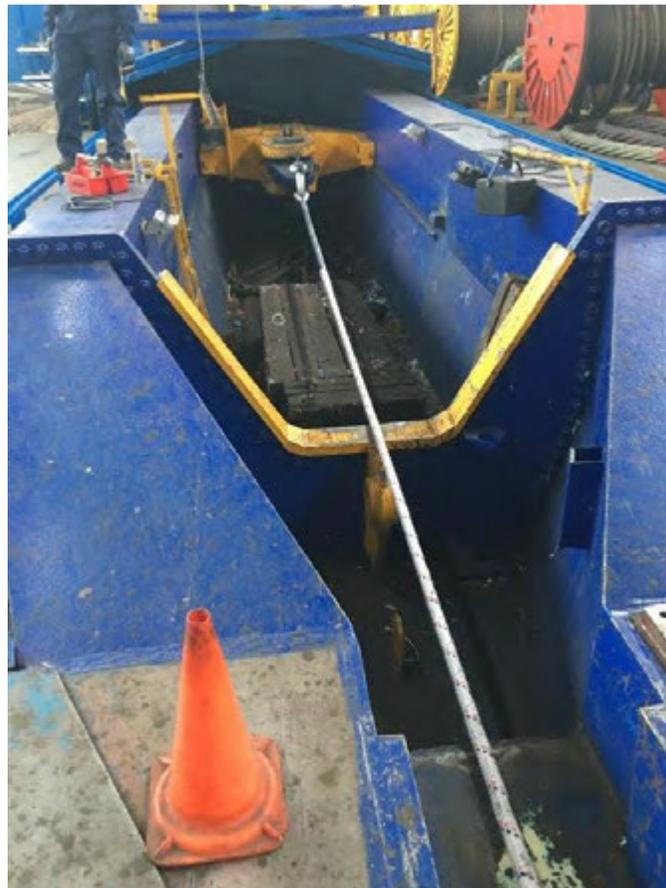
Figure 4.3.1: Rope sample 2 installed in test bed, looking towards active end.
