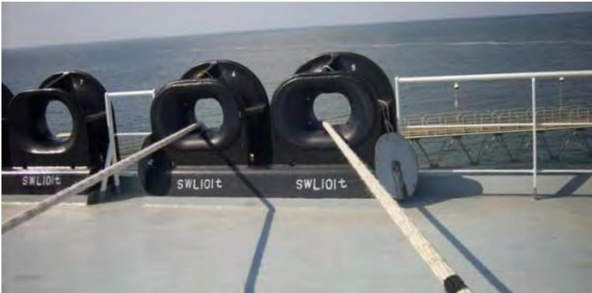
**Figure 2:** Fixed steel Panama fairleads, right, with ropes and nylon liners.
