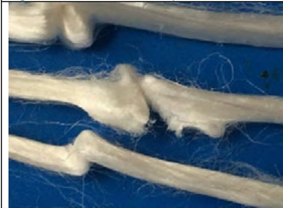
Figure 6.5 – Shore end - partial yarn failure
