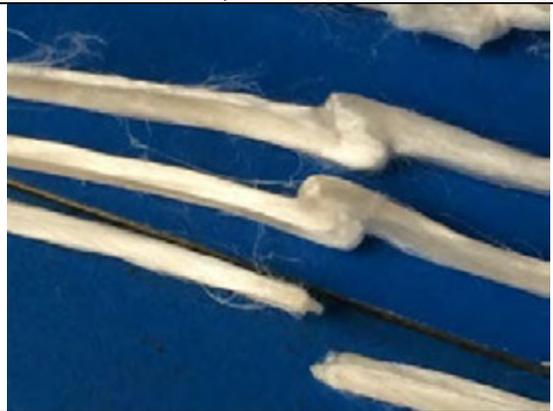
Figure 6.6 – Shore end - failed end
