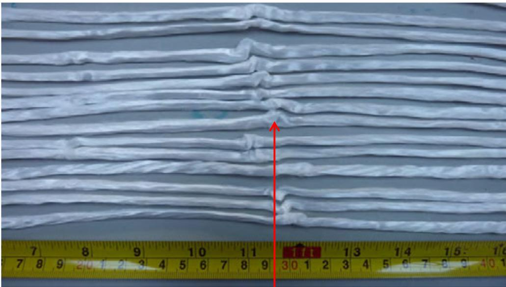
Figure 4.1.4: Sample 1, inner rope yarns, close up of severe buckles shown in figure 4.1.3
