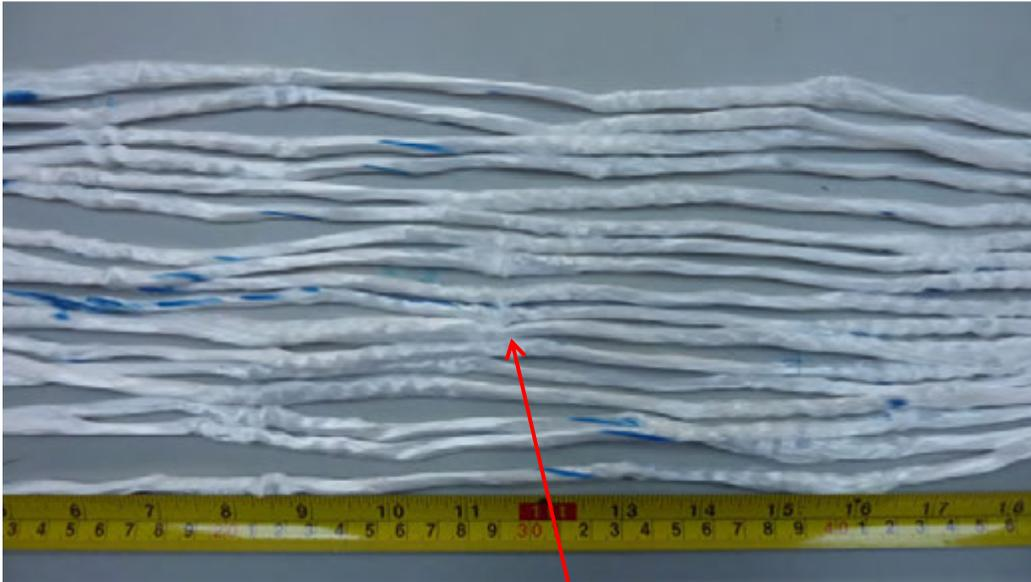
**Figure 4.1.5:** Sample 1, outer rope yarns, close up of mild buckles shown in figure 4.1.3.
