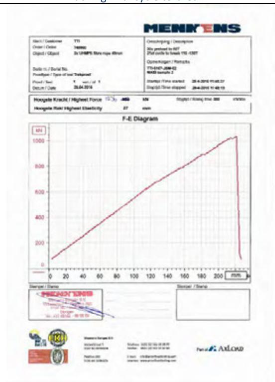
Figure 4.3.7 – Load extension curve for Sample 2 during final cycle to break
