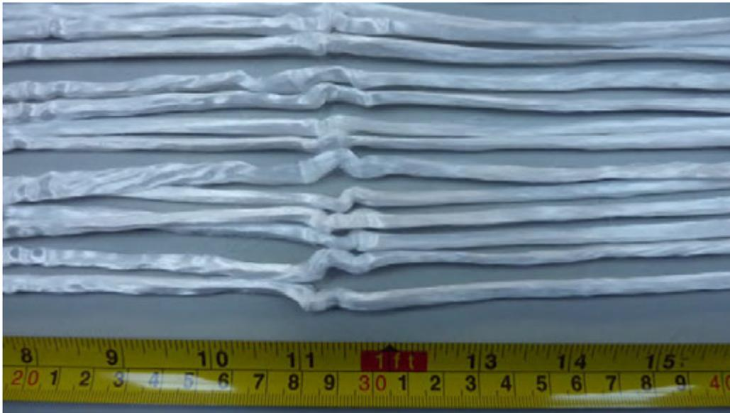
Figure 4.1.11: Sample 2, close up of severe buckling in figure 4.1.10
