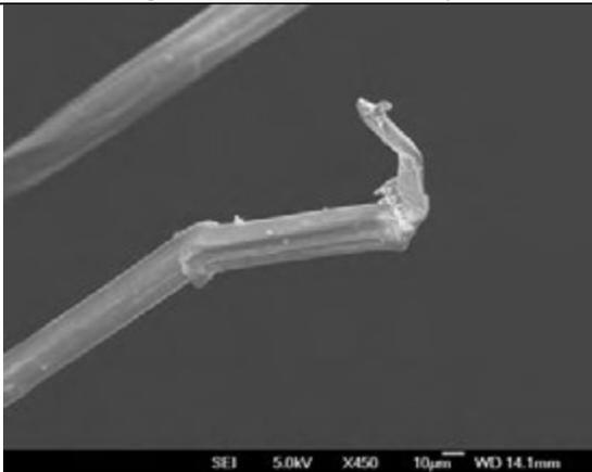
Figure 8.16 – Area A – Kinkband filament failure
