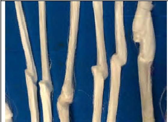
Figure 6.13 – Vessel end middle – severe kinks found but no evidence of yarn failure
