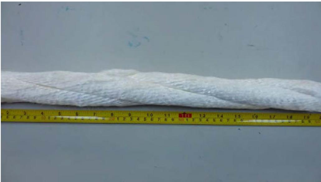
**Figure 4.1.6:** Sample 2, 3 strand subrope, very minor buckling in outer layer
