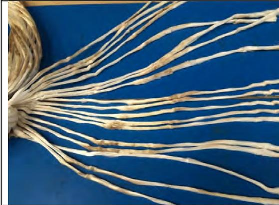
Figure 6.11 – Vessel end middle – outer yarns. All strands with similar small kinks
