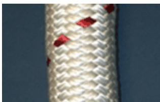
**Figure 4: Koronakis Core with Jacket**
