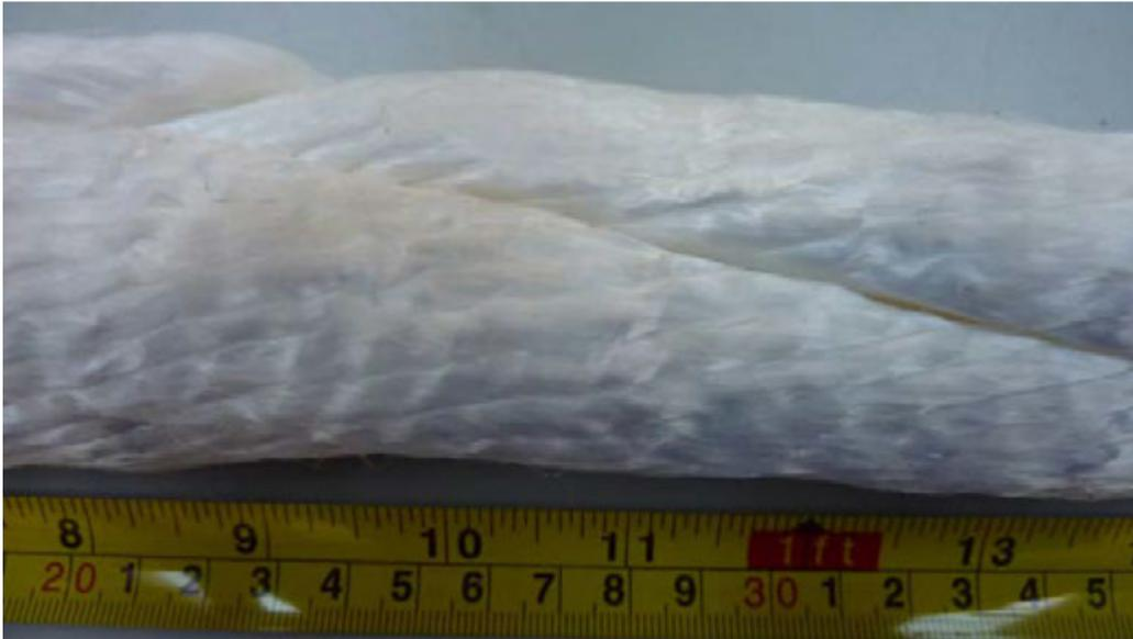
Figure 4.1.7: Sample 2, 3 strand subrope, close up of very minor buckling in outer layer
