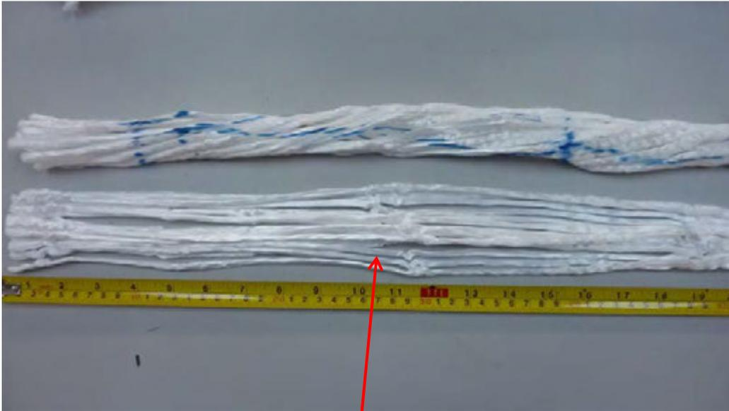
Figure 4.1.3: Sample 1, strand unlaidd to rope yarn, inner layers zero twist and severely buckled
