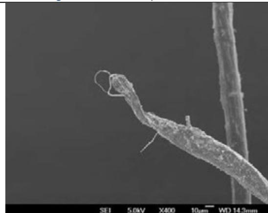
Figure 8.12 – Close up of filament failure
