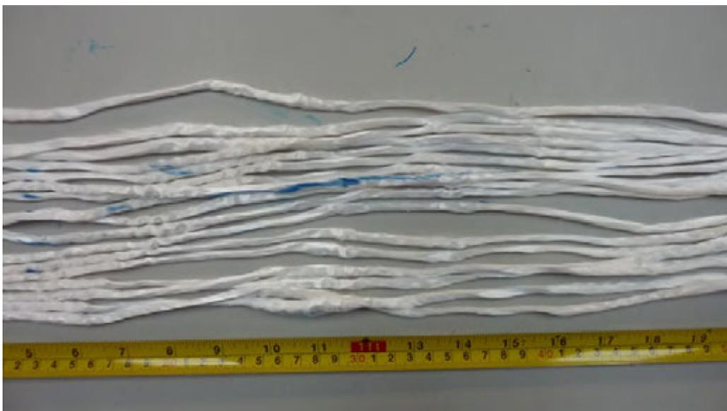
Figure 4.1.12: Sample 2, outer rope yarns, mild buckles shown in figure 4.1.9, note not all yarns buckled
