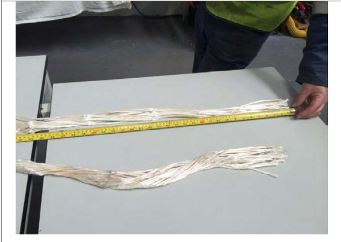
Figure 4.1.4 – Original Shore Side Sample - Kink band frequency measurement
