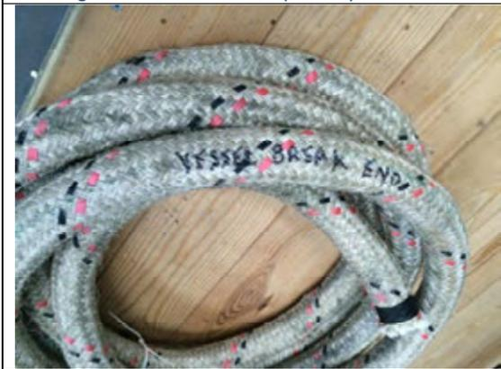
Figure 6.7 – Vessel break end
