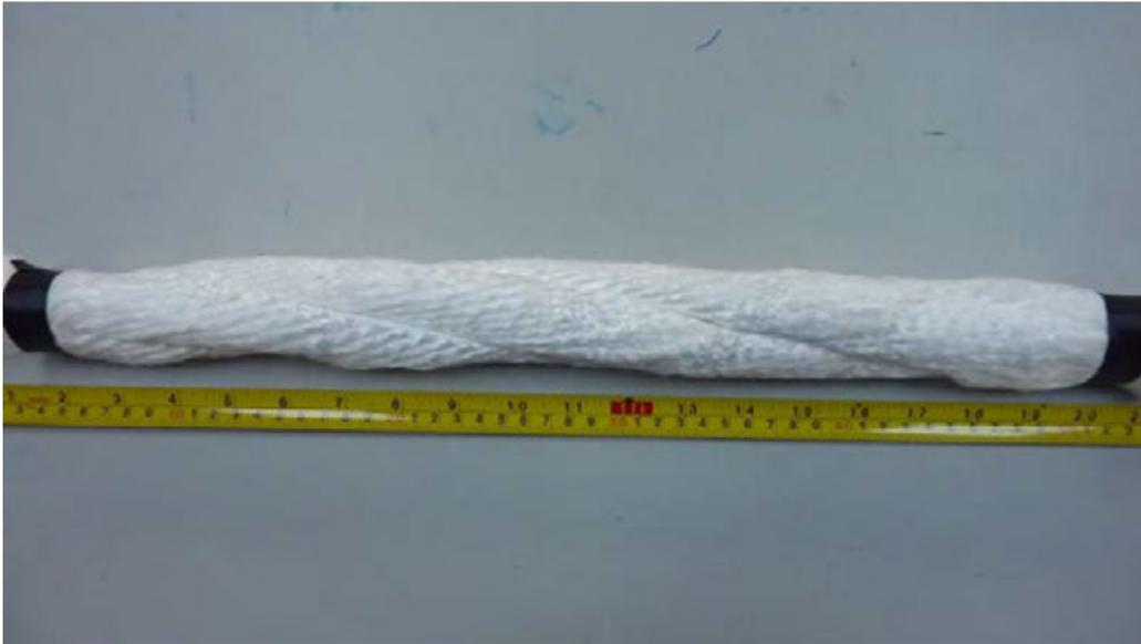
**Figure 4.1.13:** Sample 3, 3 strand subrope, very minor buckling in outer layer
