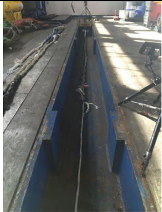
Figure 7.8 – Mooring line section following test
