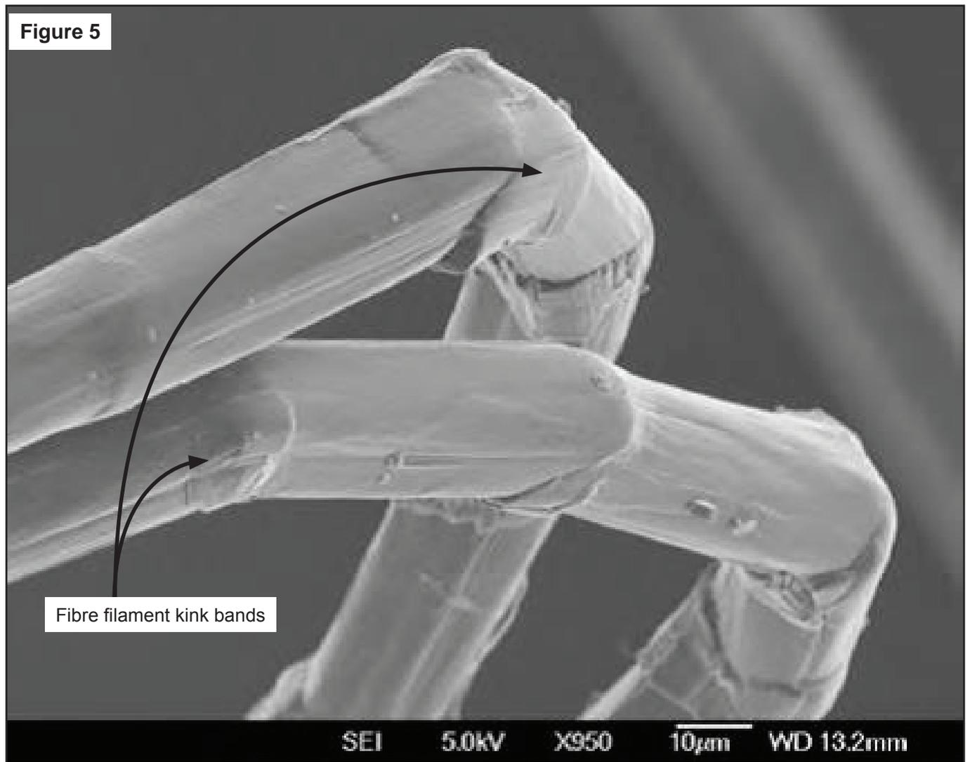
Close-fitting jackets prevent operators from visually inspecting these types of rope for core and yarn fatigue damage, and there are currently no non-destructive tests available to assess the level of fatigue degradation in fibre filaments in ropes. If it had been possible to visually inspect the load-bearing core of *Zarga's* rope, the rope yarn kinks and the broken rope yarns would have been identified.
