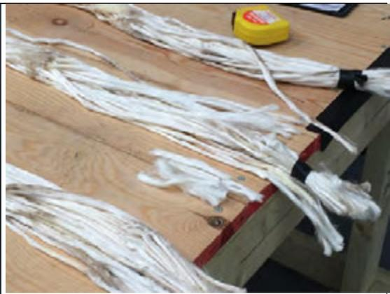
Figure 4.1.2 – Original Shore side sample - Multiple yarn failures in core yarn of one strand
