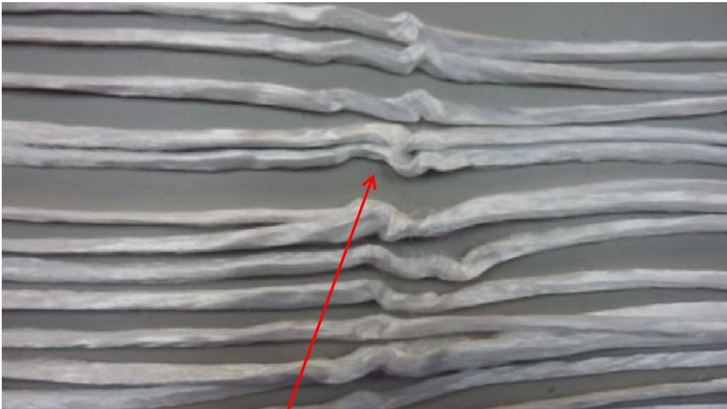
**Figure 4.1.18:** Sample 3, close up of severe buckling in figure 4.1.17
