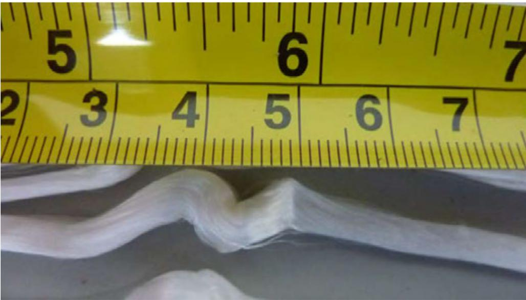
Figure 2.3. Close-up of an inner yarn buckle (Mode 4, see below) with a characteristic length of about 10mm
