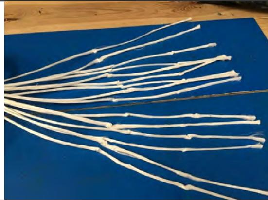
Figure 6.12 – Vessel end middle – severe kinks found in one strand
