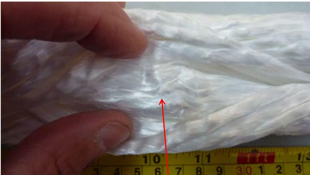
Figure 4.1.8: Sample 2, opened outer layer strand to reveal inner rope yarns, close up of severe buckling
