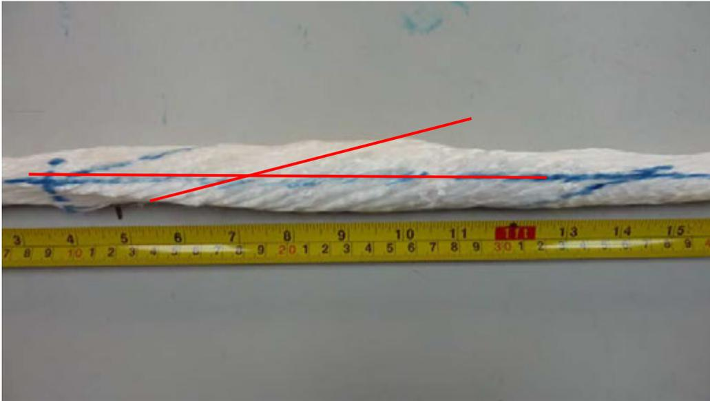
**Figure 4.1.9:** Sample 2, Strand unlaidd, very mild buckling in outer layer rope yarns, 15 degrees and pitch 255mm.
