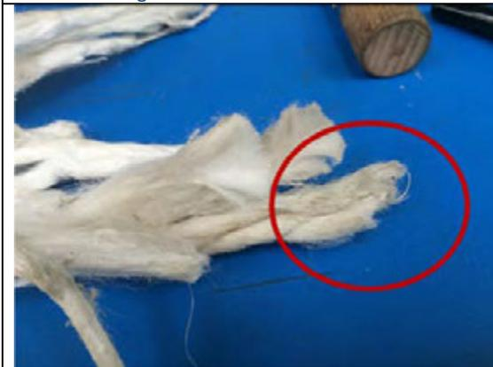
Figure 8.27 – Vessel end possible tensile failure
