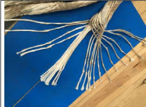
Figure 6.3 – Shore end – Outer yarns – kinks evident
