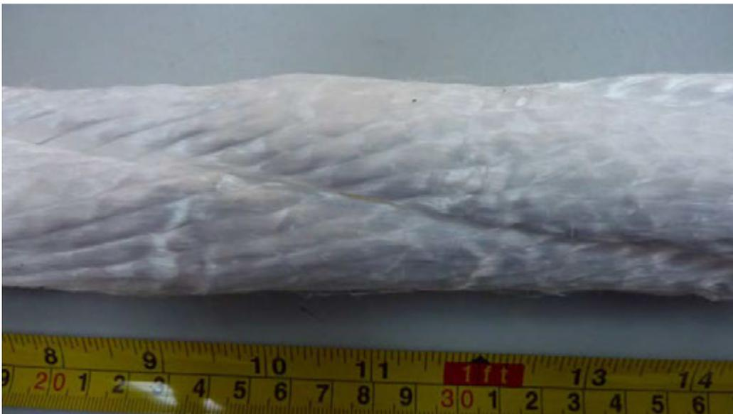
**Figure 4.1.14:** Sample 3, 3 strand subrope, close up of figure 4.1.13, very minor buckling in outer layer
