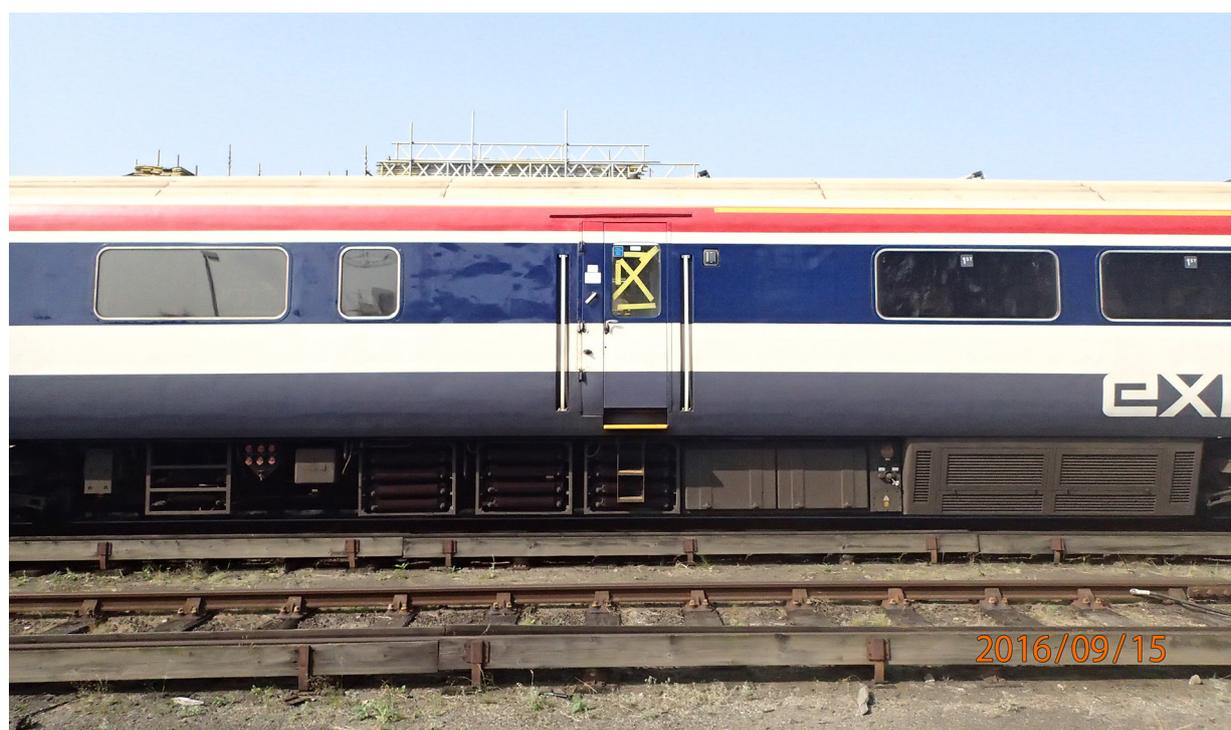
Figure 11: Class 442 unit with hazard tape applied to guard's droplight window
