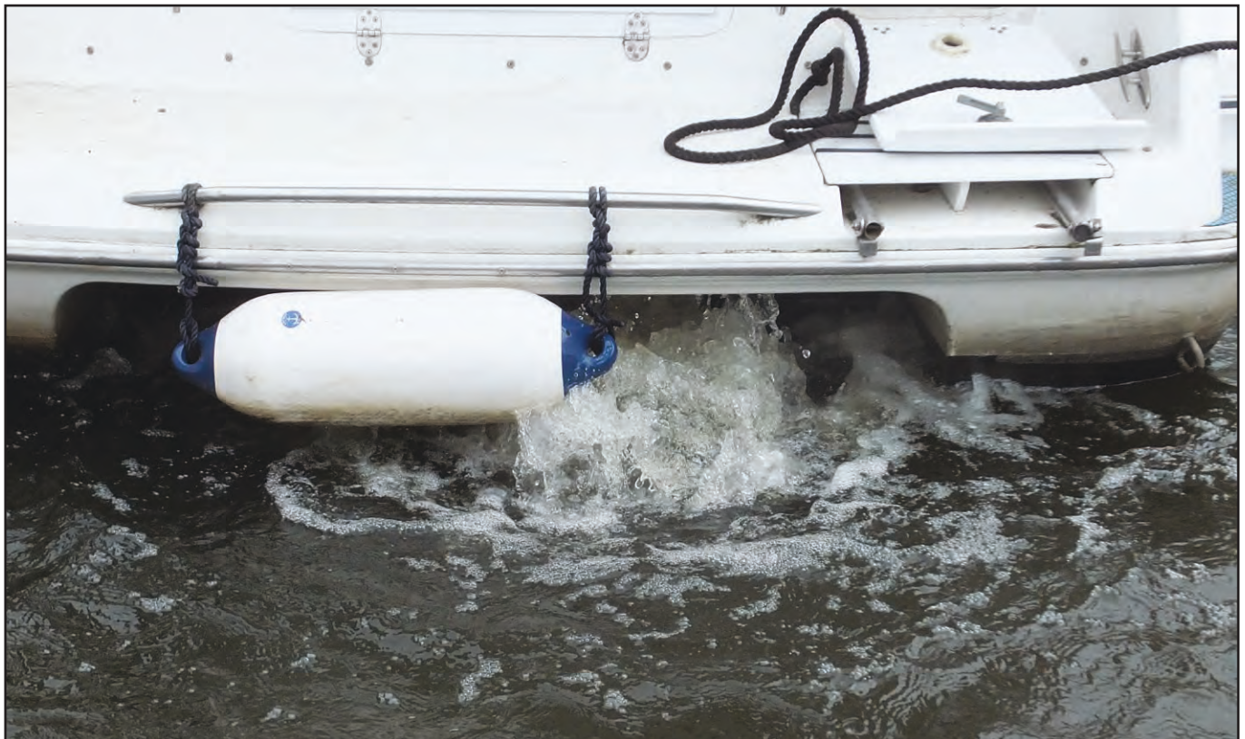
Figure 2: Wet exhaust at boat's stern
