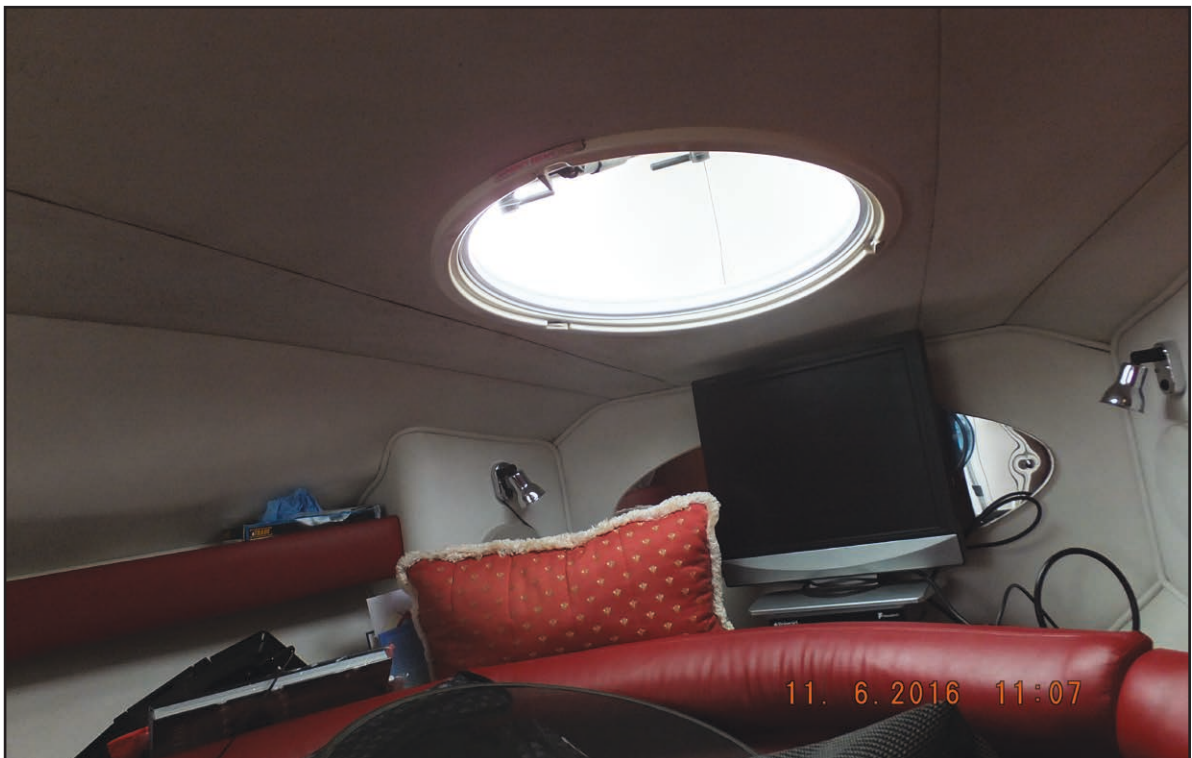
Figure 5: Forepeak cabin hatch/vent
