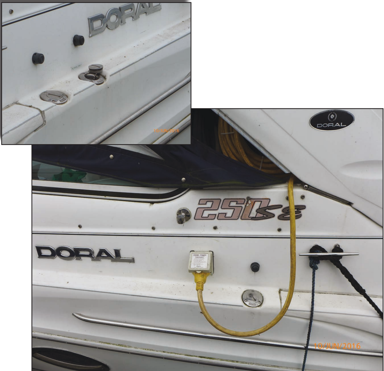
Figure 10: Shore cable and fuel tank cap
