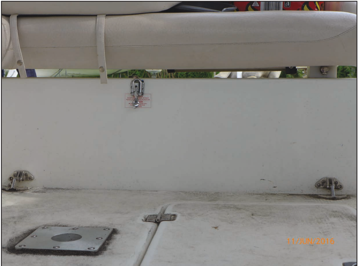
Figure 7: Gap under aft bench seat
