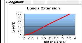
Typical working elongation (for a bedded in rope):
