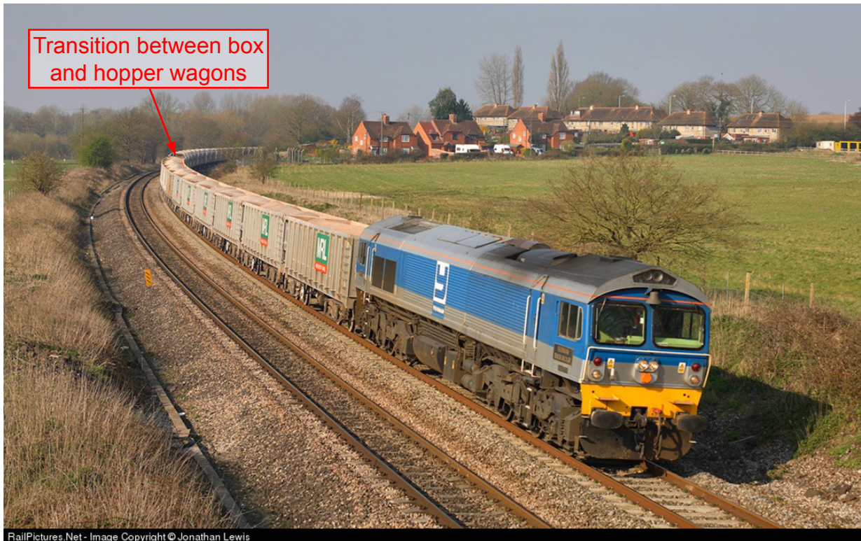
Figure 4: A train similar to 7A09. The train is formed of a mixture of box wagons (at the front of the train) and hopper wagons (image courtesy of Jonathan Lewis)
