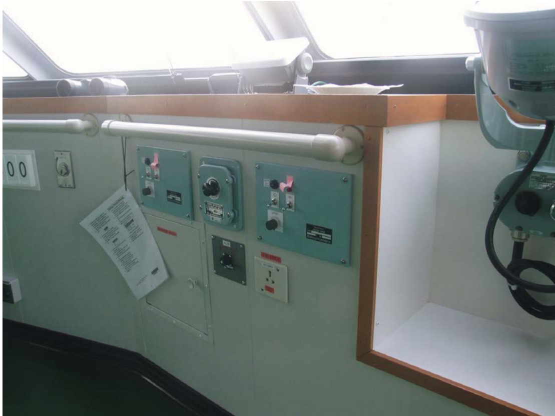
Figure 13. Pilot plug, and centreline compass repeater.
