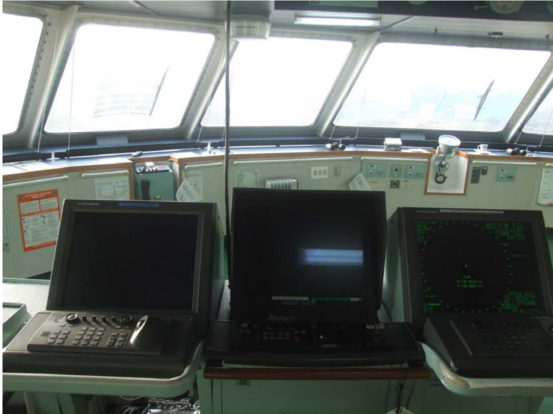
Figure 9. View fwd. from a navigating position. Note difficulty in establishing the centreline.
