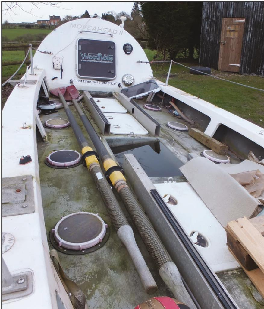
**Figure 8:** An ocean rowing boat fitted with guard wires
