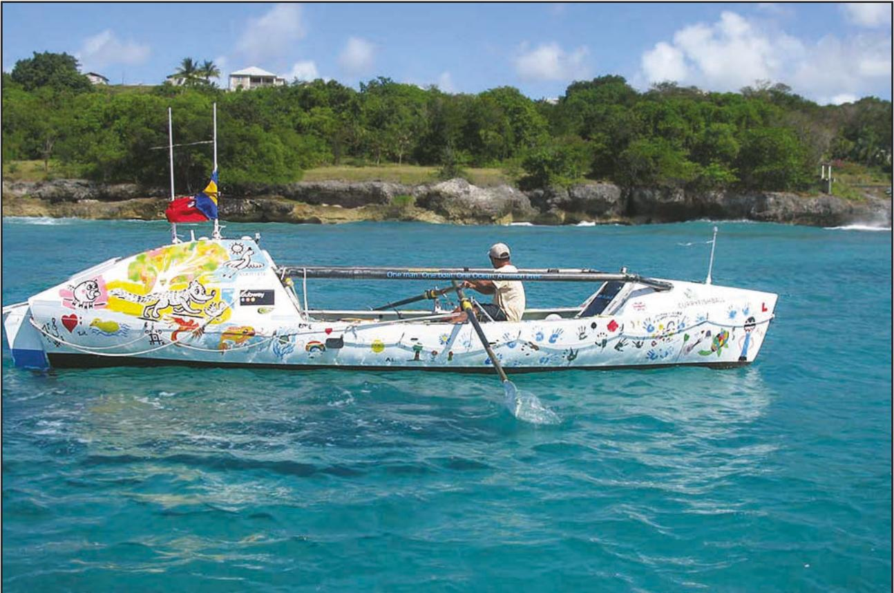
**Figure 7:** An ocean rowing boat fitted with guardrails
