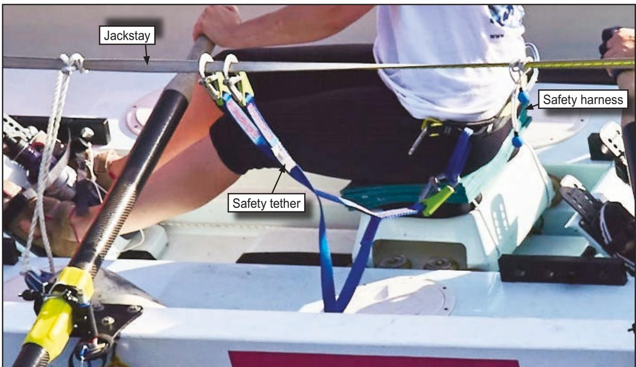
**Figure 9:** Use of a safety harness, tethers and jackstay
